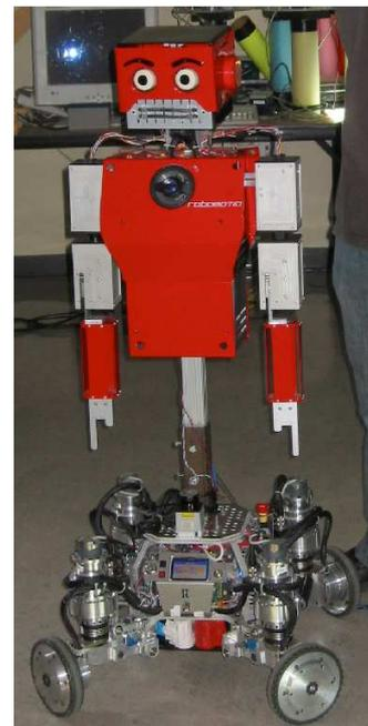
Figure 3. Reddy platform on top of AZIMUT-3 wheeled platform.
