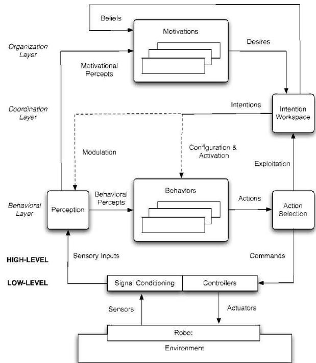
Figure 4. Hybrid Behavior-Based Architecture.
