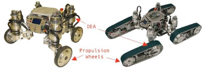
Figure 2. AZIMUT-3 in its wheeled configuration (left) and its tracked configuration (right).
