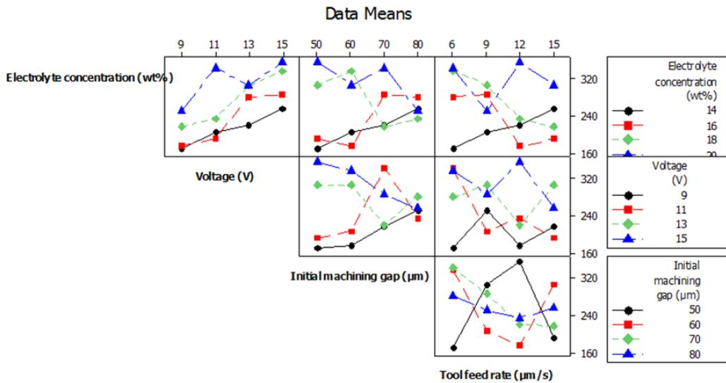
Figure 3. Interaction plot of factors for radial overcut.
