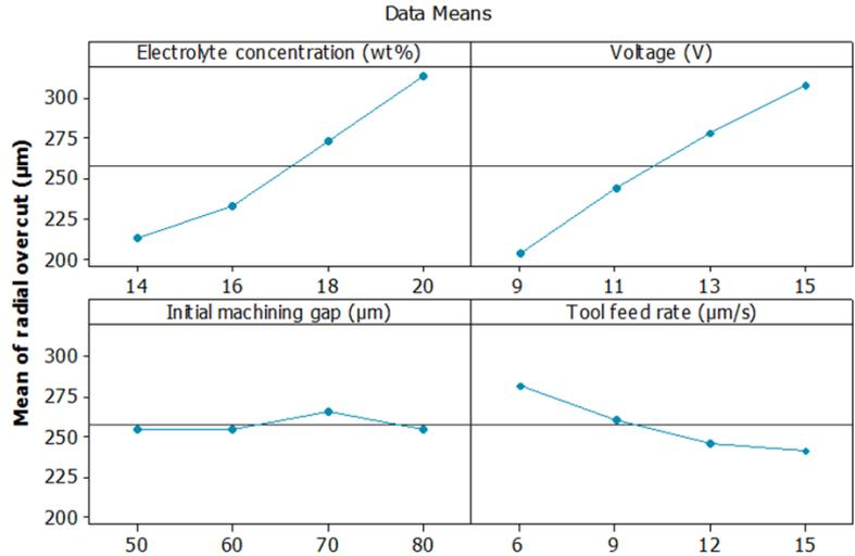
Figure 2. Main effect plot of the process parameters on radial overcut.
