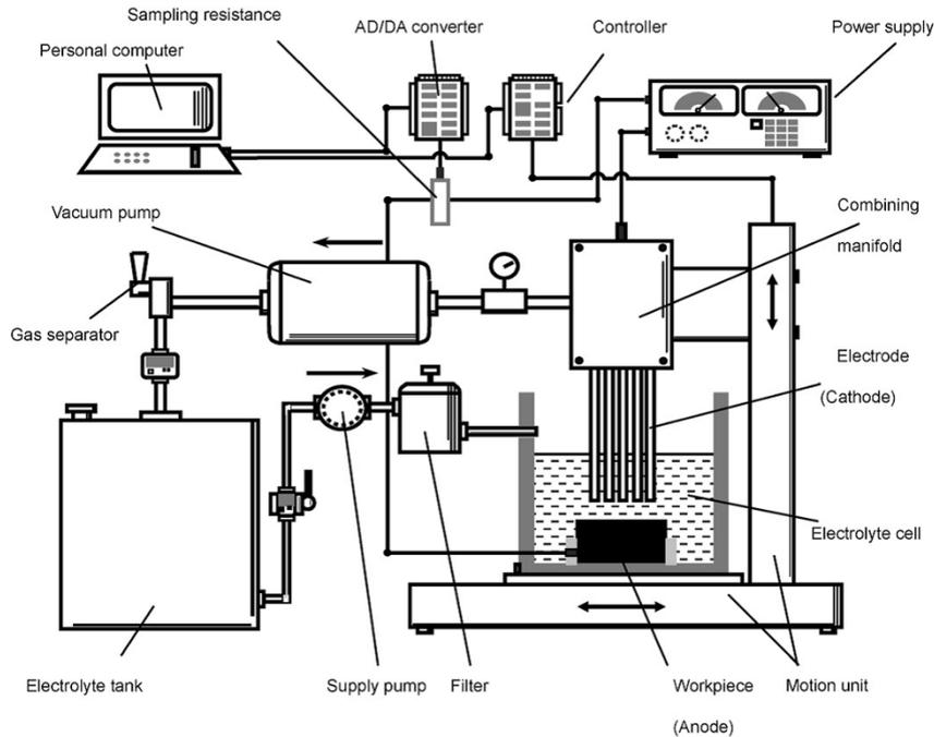
**Figure 1.** Schematic diagram of the experimental set-up [6].
