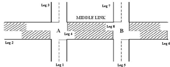
Figure 1. An arterial with two intersections
