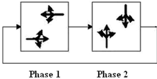
**Figure 3.** Phase diagram for two-phase signal
