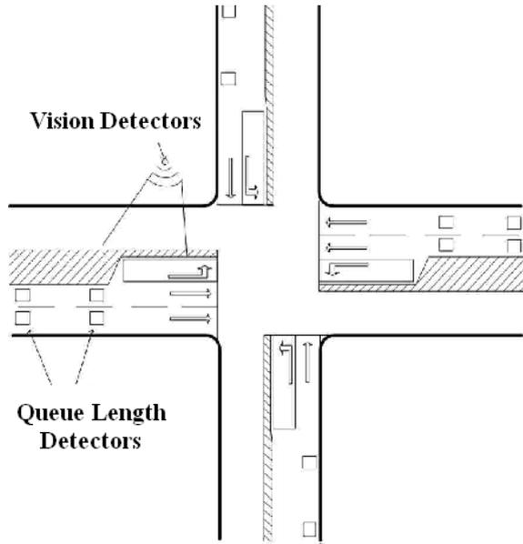
**Figure 2.** An intersection with typical detectors and lane configuration
