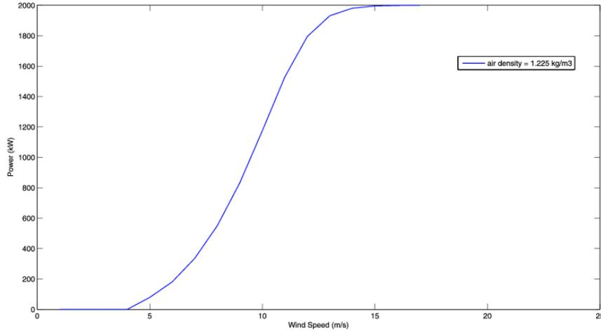
**Figure 2.** Example of power curve.
