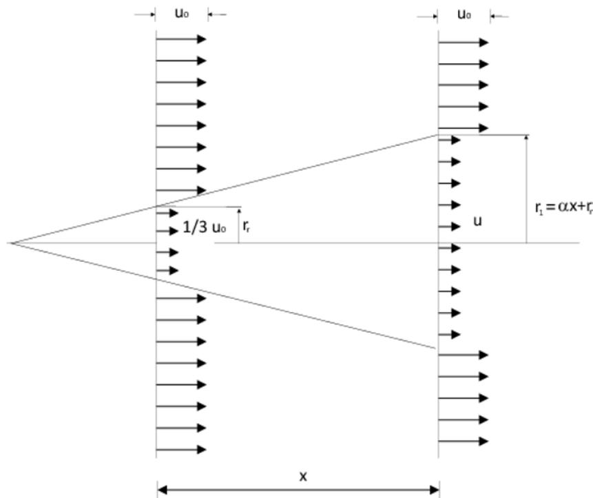
**Figure 1.** Schematic of a wake model.
