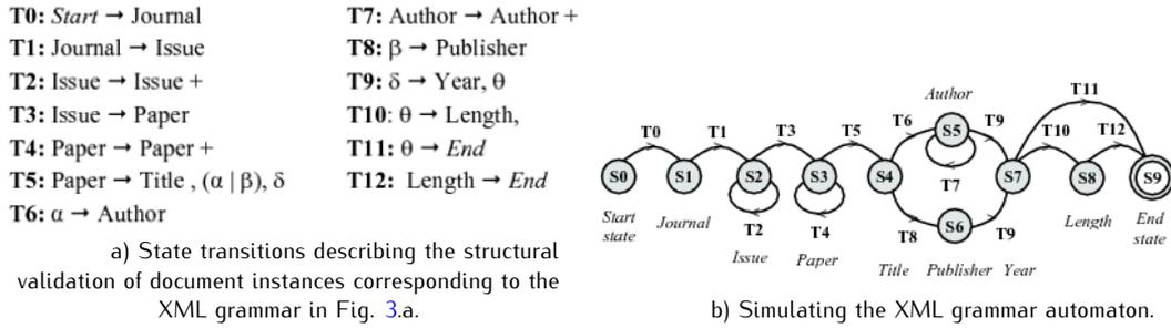
**Figure 4.** XML grammar automaton to perform document validation.
