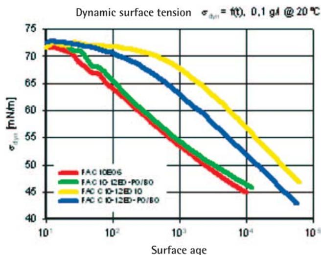
**Figure 9** Dynamic surface tension data (picture credit: H. L. Möhle, Kolb)
