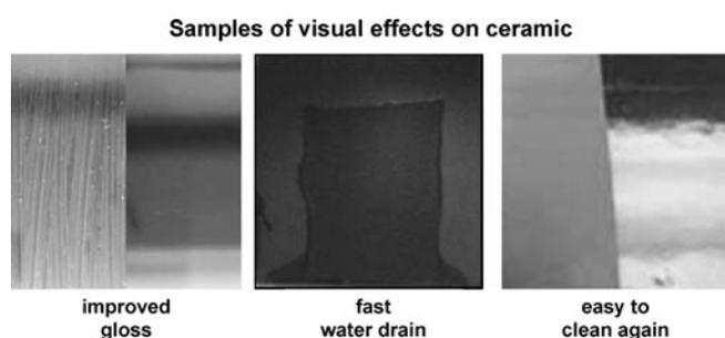
**Figure 1** Surface Modification: Samples of visual effects on ceramic (picture credit: *T. Albers*, Cognis)
