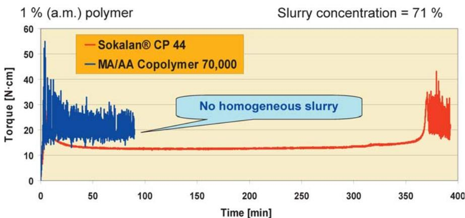
Figure 5 Viscosity progression in a zeolite-based detergent slurry (picture credit: H. Gumbel, BASF)
