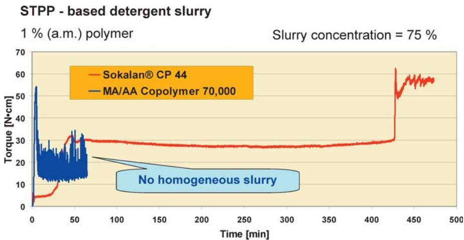
Figure 6 Viscosity progression in a STPP-based detergent slurry (picture credit: H. Gumbel, BASF)
