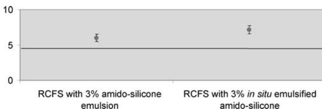
Figure 4 Softness performances of in-situ emulsified amido-silicone material versus the postaddition of emulsion of the same amido-silicone material. The black line represents the reference got when using the simple RCFS (picture credit: St. Ugazio, Dow Corning)
