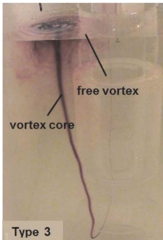
Fig. 2. Setup of a surface vortex [5]
