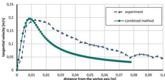
Fig. 7. Calculated and measured tangential velocity distribution (0.44 m/s)
