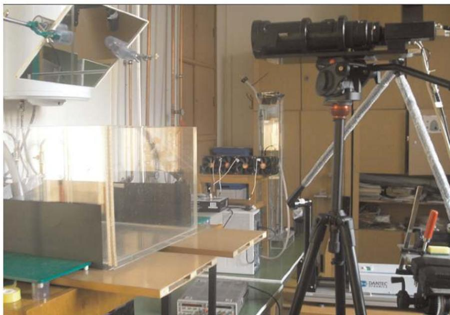
Fig. 3. Setup of the experiment and the PIV camera [8]
