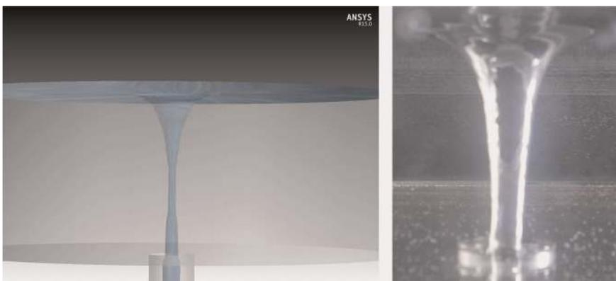
Fig. 5. Calculated (left) and the during the experiment observed surface vortex (right) [8]
