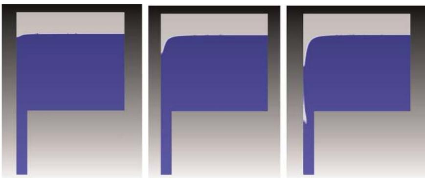
Fig. 6. Phase boundary at different intake velocities, blue: water and white: air (0.1, 0.25, 0.44 m/s)
