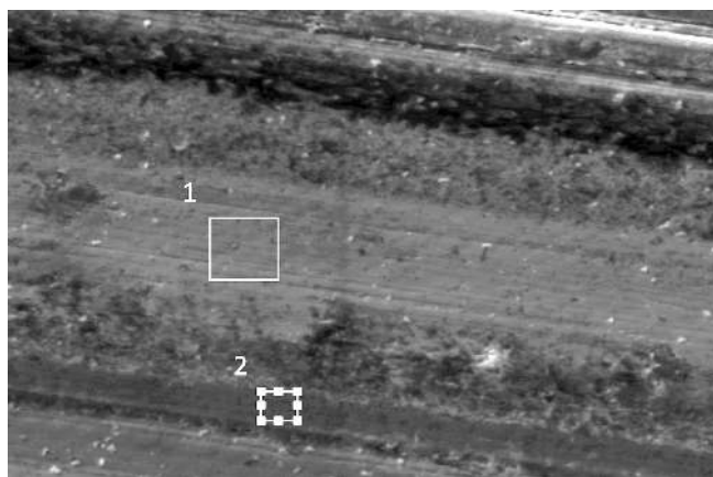
Fig. 6. Scanning electron microscopy image showing the wear scar of an Al 6061 ball after wear testing in lubricant L7-FFO.
