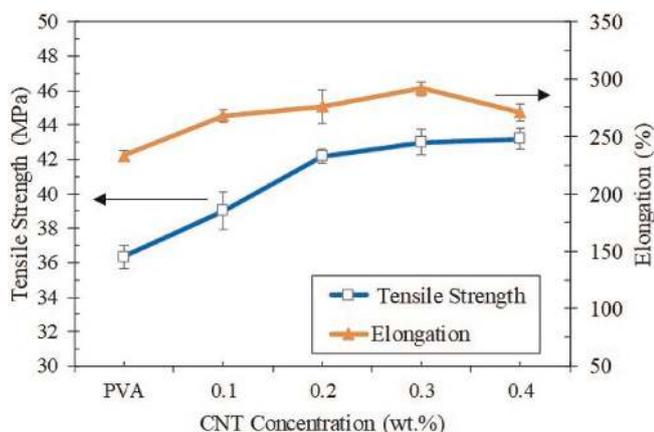
Fig. 4. Effect of CNT concentration on the mechanical properties of nanocomposite film.
