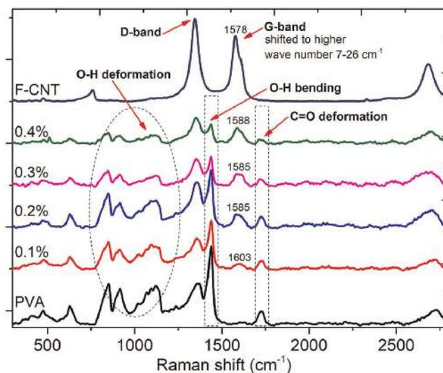
Fig. 8. Raman spectroscopy for nanocomposite film.
