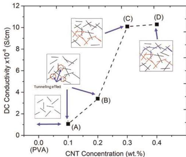
Fig. 6. DC electrical properties of nanocomposites of interest and schematic for CNT pathways within the nanocomposite film.
