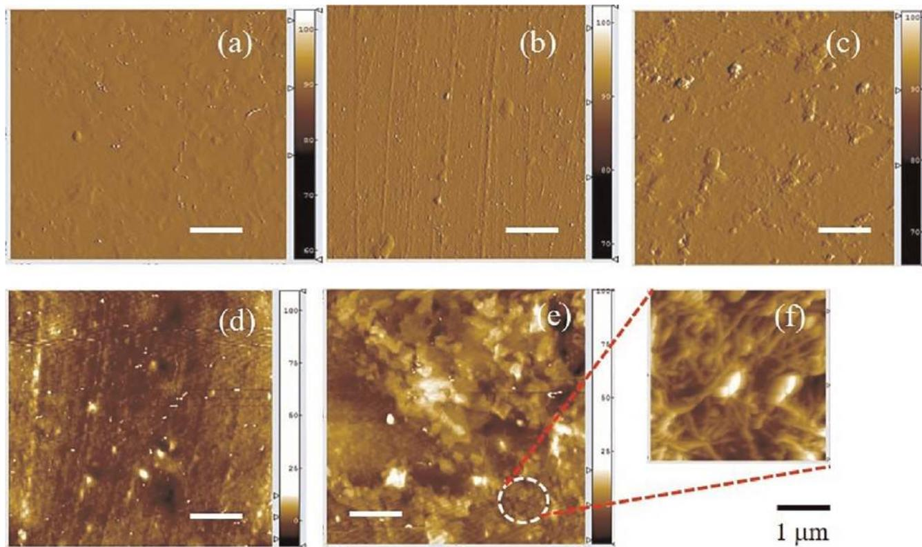
Fig. 5. AFM images of PVA and nanocomposite film at various concentrations of MWCNT (a) PVA Film, (b) 0.1 wt.%, (c) 0.2 wt.%, (d) 0.3 wt.%, (e) 0.4 wt.%, (f) Bundled nanotube.
