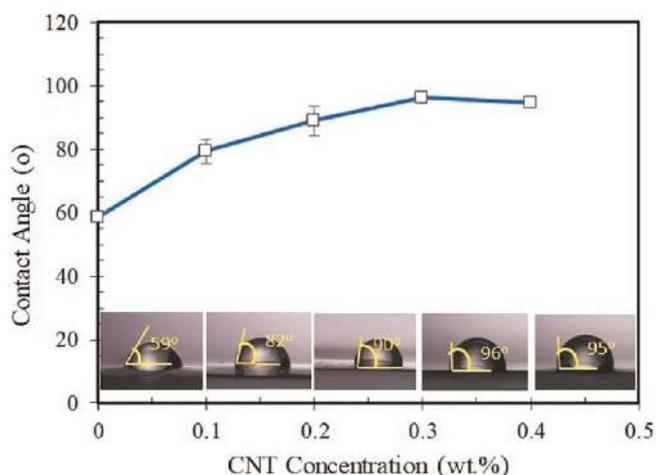
Fig. 7. Hydrophobicity of nanocomposite film.
