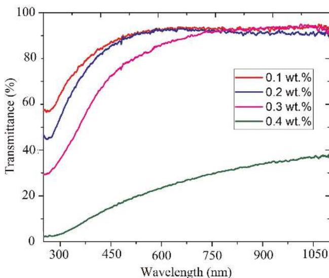
Fig. 2. Effect of CNT concentration on film transparency.
