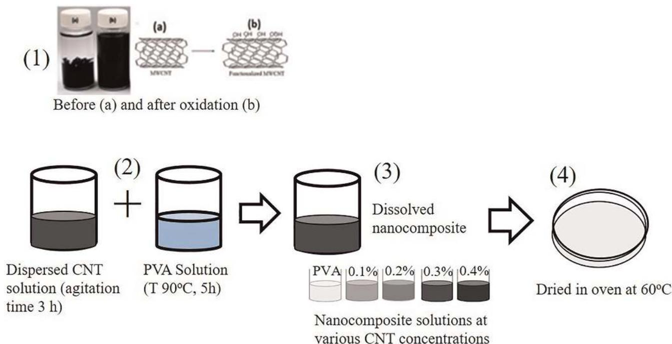
Fig. 1. Fabrication of nanocomposite film.
