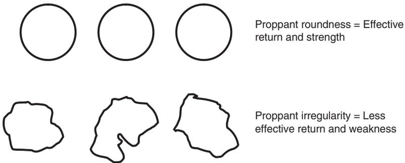
Figure 2 Proppant shape. Courtesy of the authors.
