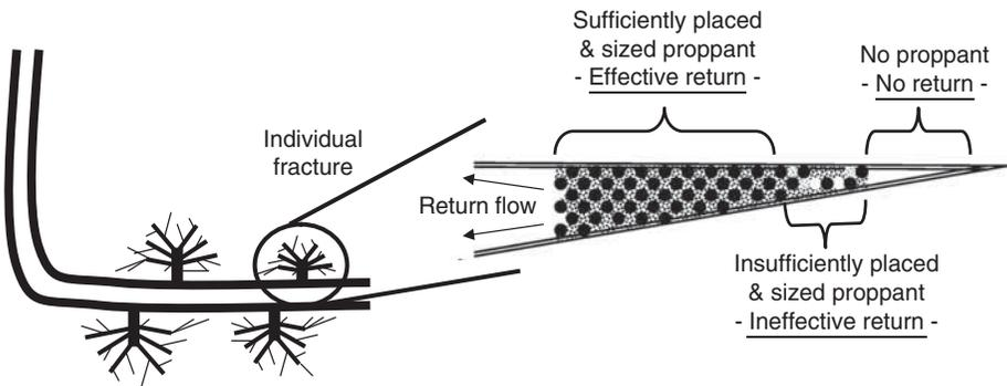
Figure 1 Proppant size and placement. Courtesy of the authors.
