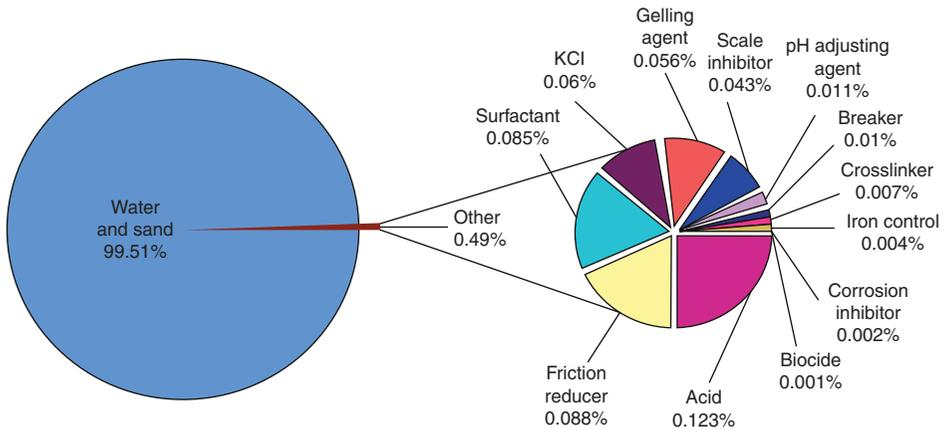
**Graph 1** Volumetric percentages of additives in fracturing fluids from Modern Shale Gas Development in the United States.
