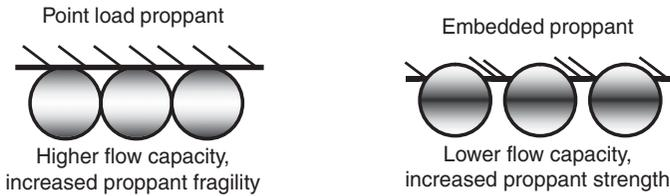
**Figure 3** Proppant hardness. Courtesy of the authors.
