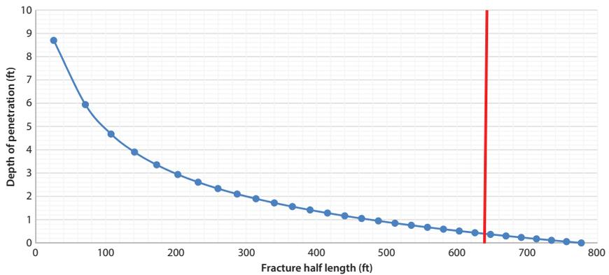
**Plot 2** Fracture half-length vs. depth of penetration.
