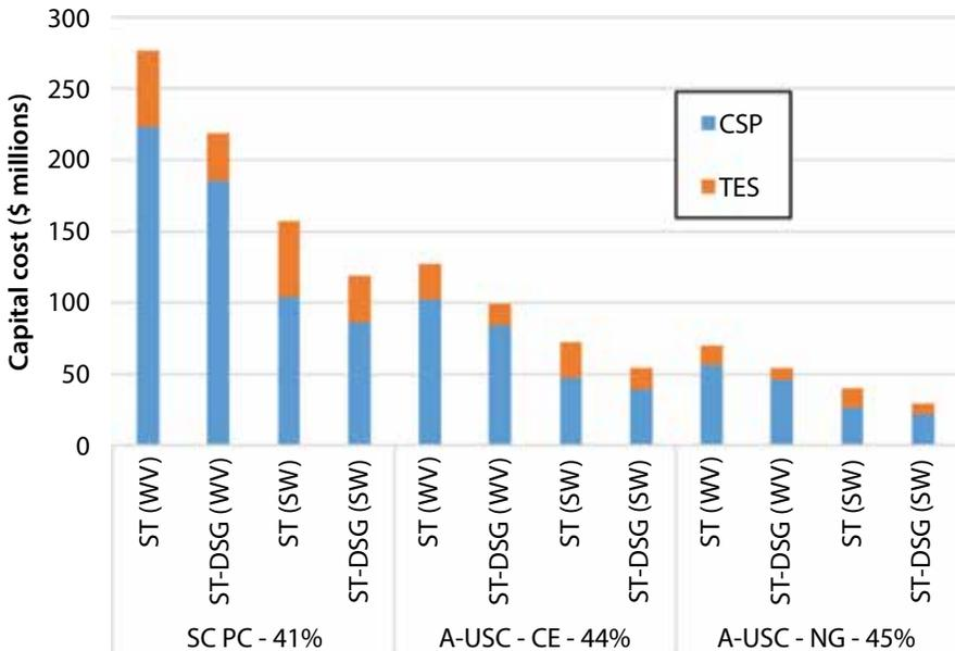
**Figure 3** Concentrating solar power and thermal energy storage installed cost breakdown.
