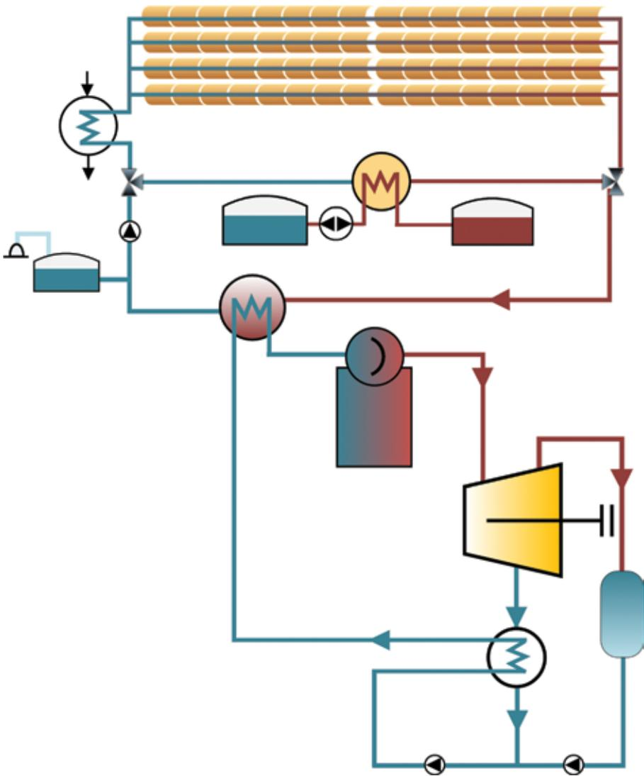
**Figure 1** Solar aided feedwater heating system with mineral oil heat transfer fluid.
