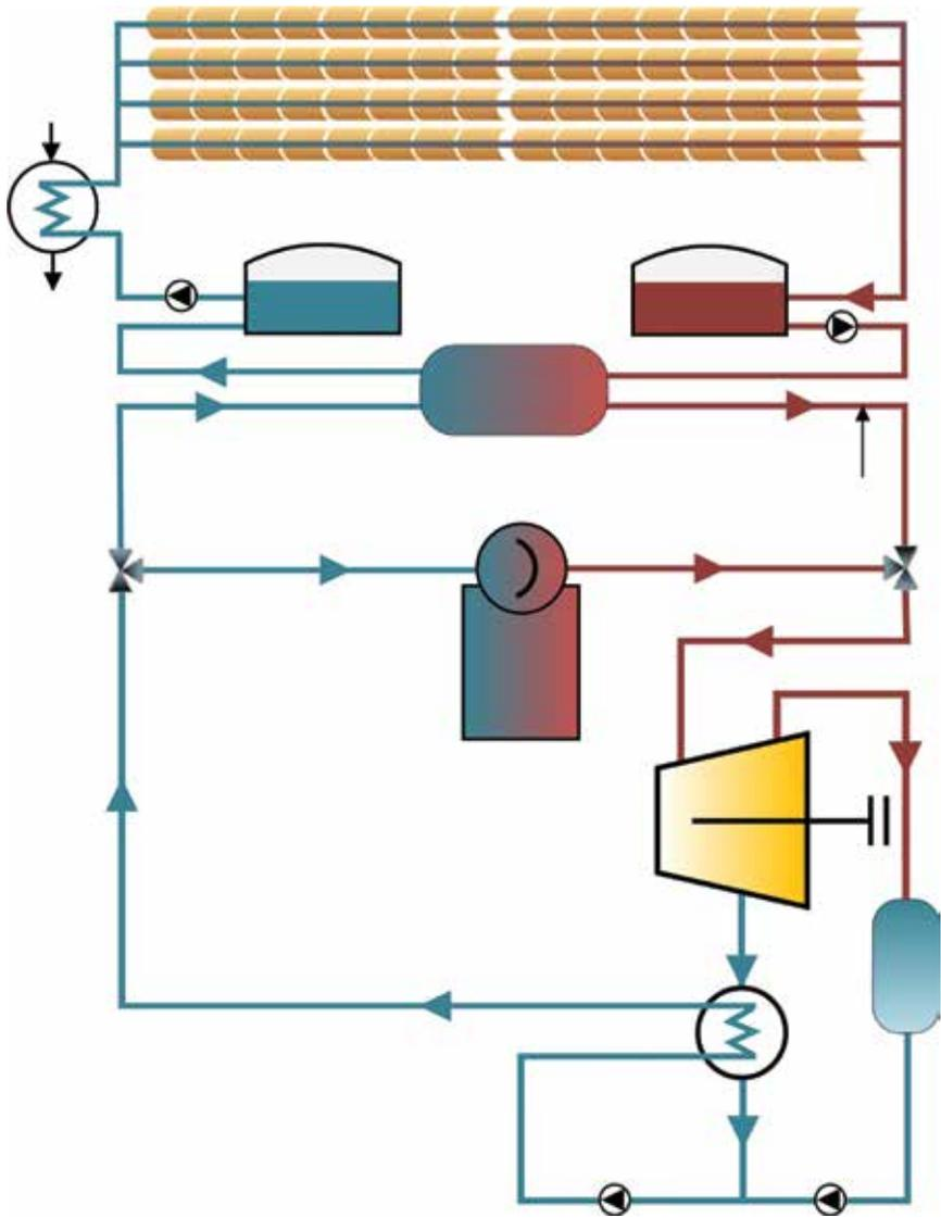
**Figure 2** Solar aided feedwater heating system with molten salt heat transfer fluid.
