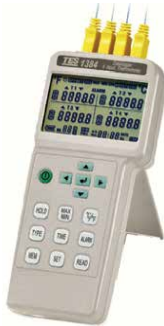
Figure 7 The data logger (TES1384) used to record the thermocouple readings.
