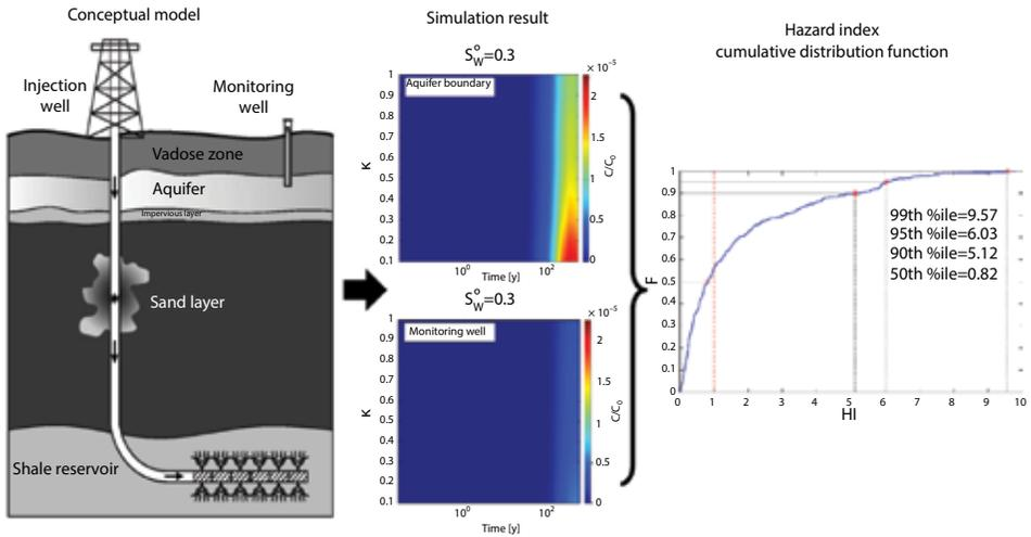
**Figure 5** Numerical Modeling to Quantify Risk Factors for Water Contamination Associated with Hydraulic Fracturing, Jabbari et al (2016).
