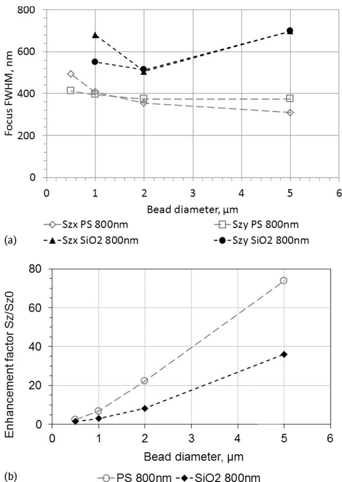
**Fig. 7.3:** Focus FWHM diameter (a) and enhancement factor (b) beneath a microsphere particle submerged in water vs. particle size (wavelength  $\lambda = 800$  nm). The focal diameters are determined in the planes of highest enhancement. The connecting lines are a visual aid only.
