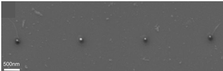
**Fig. 7.10:** Line of voxel generated by irradiating a 3.5  $\mu\text{m}$  polystyrene microbead in NOA84 photopolymer. Average voxel diameter is  $83 \pm 11$  nm. Image adopted with permission from [41].
