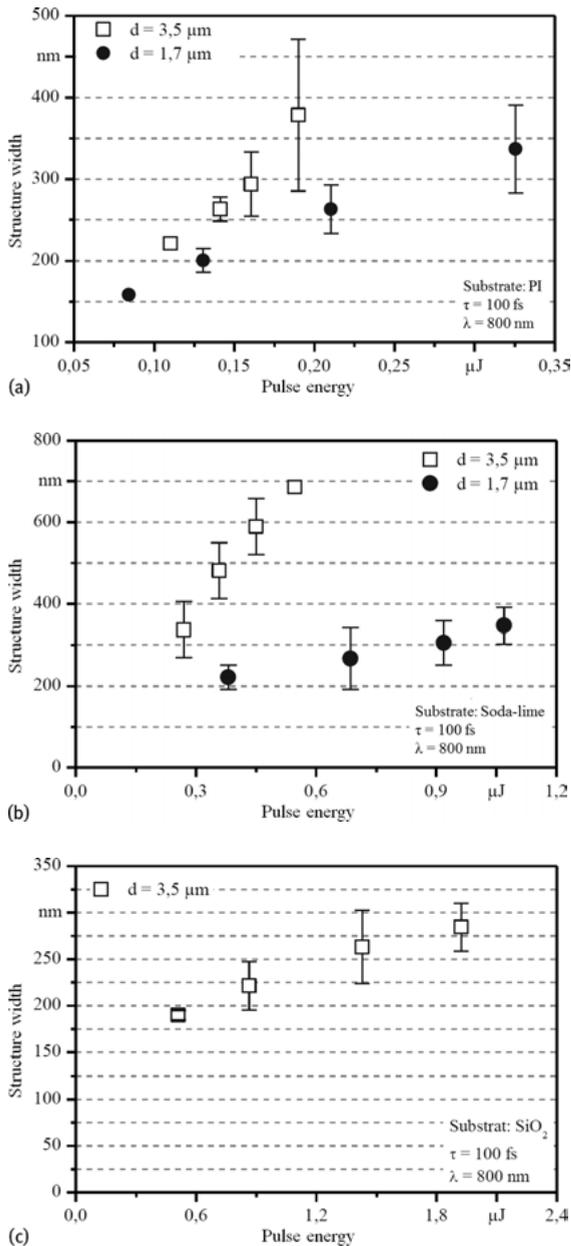
**Fig. 7.9:** Variation of dot-like structure size on polyimide coating (a), soda lime glass (b), fused silica glass (c) for different laser pulse energies. The laser wavelength is 800 nm and the pulse duration 100 fs. The focusing polystyrene particle sizes are 1.7  $\mu\text{m}$  and 3.5  $\mu\text{m}$  in diameter except for the fused silica substrate; here only 3.5  $\mu\text{m}$  beads have been used.
