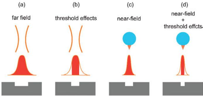
**Fig. 7.1:** Feature size reduction in laser based structuring: (a) restriction of feature size by diffraction in the far-field; (b) reduction of feature size by utilization of threshold effects; (c) reduction of feature size by utilization of near-field effects; and (d) further reduction of feature size via combination of near-field and threshold effects. Adopted with permission from [42].
