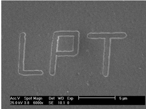
**Fig. 7.8:** SEM microphotograph of nanostructures on polyimide (EPO-Tek P1011). Process parameters:  $2\ \mu\text{m}$  SiO<sub>2</sub> microsphere irradiated with  $\lambda = 532\ \text{nm}$ ,  $\tau = 10\ \text{ps}$ , pulse frequency  $f = 500\ \text{Hz}$  and fluence  $F = 8\ \text{mJ}/\text{cm}^2$  laser beam. Image adopted with permission from [28].
