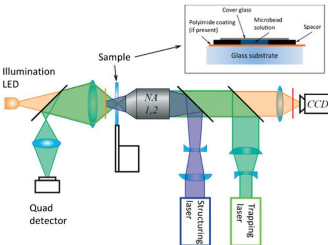
**Fig. 7.6:** Experimental setup of OTAN. Green path – optical trapping subsystem incorporating either 532 nm or 1064 nm cw laser; purple path – structuring arm which can employ either 800 nm 100 fs, 400 nm 100 fs, or 532 nm 10 ps laser pulses; light orange path – imaging subsystem used for structuring process visualization. A typical test sample is schematically shown in the insert.
