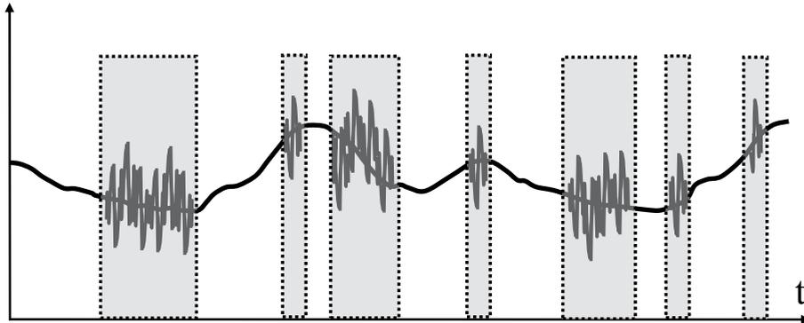
**Fig. 11.3:** Record of an instrument in a correct working condition that produces a time series with areas in which the signal to noise ratio is very low. In those sections, indicated by a gray rectangle, it is not possible to recover the signal and these pieces of the record must be removed.
