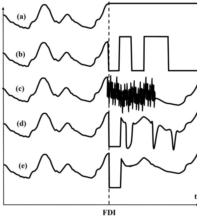
**Fig. 11.1:** Some failures beginning at FDI are observed in the data recorded: (a) the instrument begins to record a constant value; (b) data alternates between zero and out of scale; (c) noise appears preventing the signal from being rescued; (d) the instrument measures intermittently because of random failures; (e) there is a circumstantial cause producing a partial loss of data.
