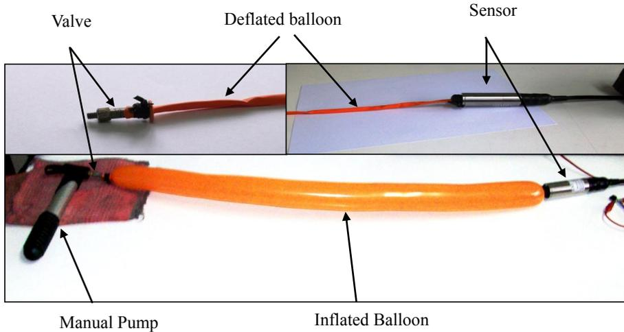
**Fig. 11.7:** Setup for testing a pressure sensor dynamically. An elastic cylinder (orange balloon) was connected to the sensor (top right) and to a valve (top left). The balloon is inflated through the valve by means of a manual pump.
