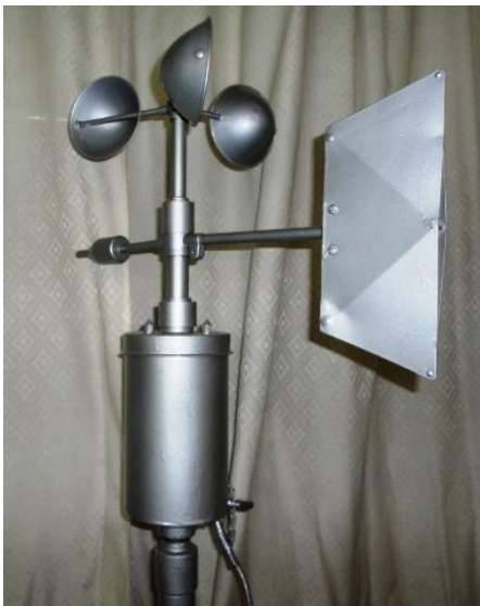
Fig. 7.3: Robust cup anemometer for use in Antarctica made of metallic parts. (Photograph courtesy of Ricardo Zuazquita, Naval Hydrographic Service of Argentina).
