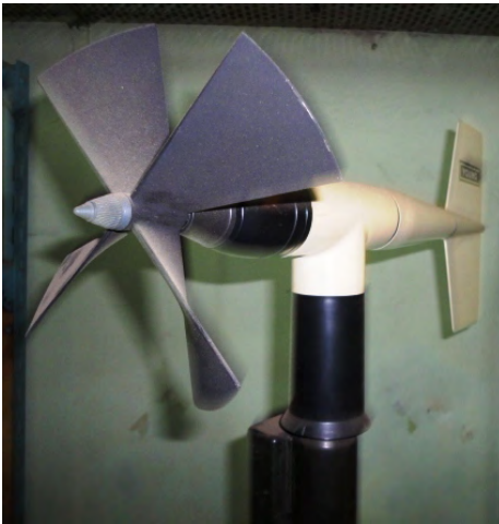
Fig. 7.1: Aerovane anemometer. (Photograph courtesy of Ricardo Zuazquita, Naval Hydrographic Service of Argentina).
