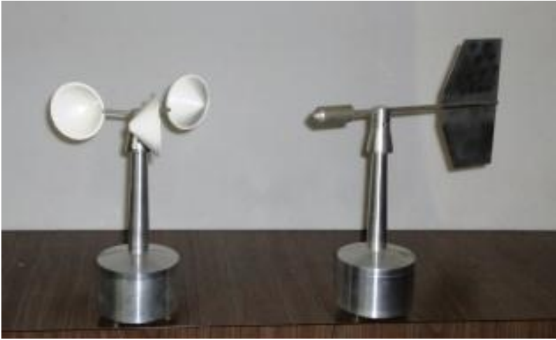
Fig. 7.2: (Left) Cup anemometer. (Right) Wind vane. (Photograph courtesy of Ricardo Zuazquita, Naval Hydrographic Service of Argentina).
