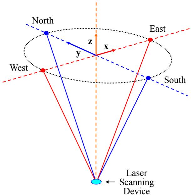
**Fig. 8.15:** The system shown in Figure 8.14 is rotated for the beam to describe an inverted cone with a vertical axis. The small dots represent the range gates (spatial cells) where the wind radial components are measured to be later converted into wind components along the  $x$ ,  $y$  and  $z$  directions.
