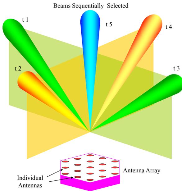
**Fig. 8.10:** An example of a RWP. The hexagon represents the antenna array and the circles the individual antennas. Each antenna is an electrical device which produces an electromagnetic wave. The beamforming of these individual waves produces the five sequential beams.
