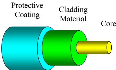
Fig. 8.1: Fiber optic components.
