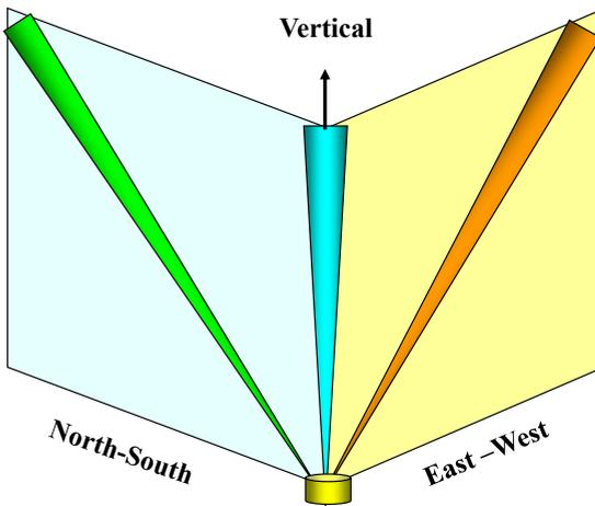
**Fig. 8.9:** Schematic of a three-beam configuration SODAR.
