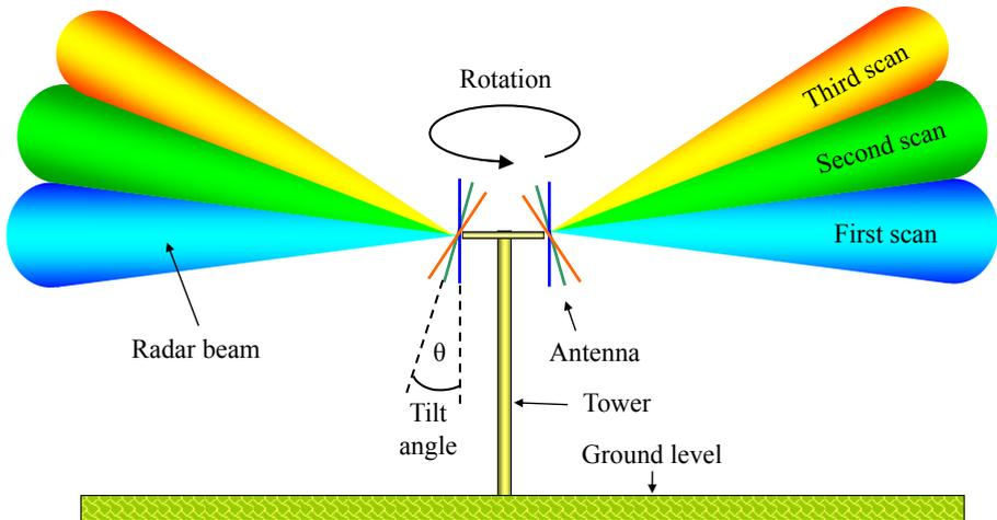
**Fig. 8.16:** The antenna rotates and the beam scans the atmosphere. After the first complete rotation the antenna is tilted and a second rotation begins. Each scan of the beam is shown with a different color.
