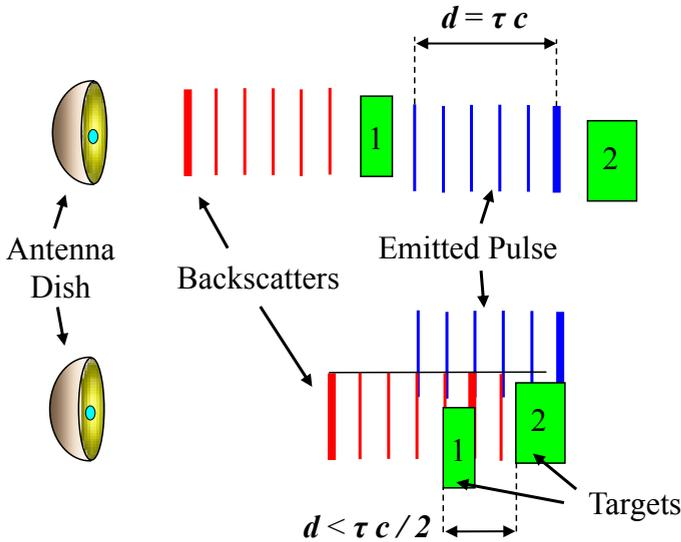
**Fig. 8.6:** Range resolution. The vertical parallel lines represent the radar wave fronts; the first wave front is shown thicker and a pulse is represented by six lines. In the upper part of the figure, the pulse is completely backscattered by the first target before the pulse arrives at the second target. In the lower figure the targets are closer to each other and the first target is scattering the fifth wave front while the second target is already scattering the second wave front.
