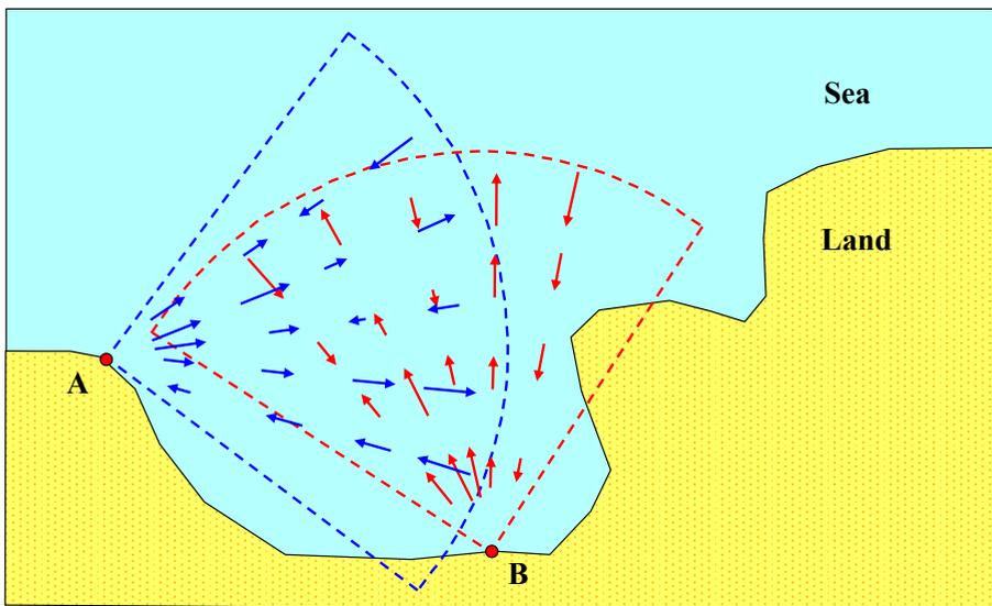
**Fig. 8.18:** The circles A and B indicate the shore installation of two radar (A and B). The dashed lines indicate the sea surface area covered by both radar systems. The arrows indicate currents measured by each of the radar. They must be composed to obtain the final current velocity field.
