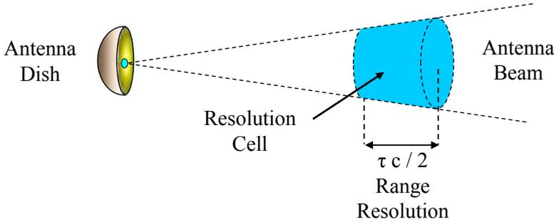
**Fig. 8.7:** The range resolution and the beamwidth of the antenna define a volume that we will call the resolution cell. The shorter the pulse width  $\tau$  and the narrower the beamwidth the smaller is the volume of the cell and the higher the ability to detect smaller targets. Thus smaller cells result in higher spatial resolution.
