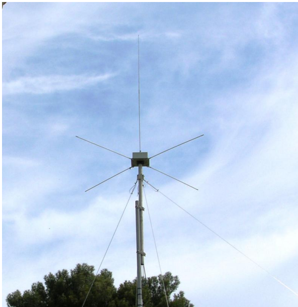
Fig. 8.20: Pole with CODAR antennas (Courtesy of Andrea Mazzoldi CNR, Italy).
