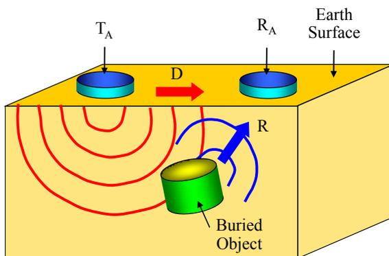
**Fig. 8.21:** A pulse is radiated by the transmitting antenna ( $T_A$ ); the receiving antenna ( $R_A$ ) will collect pulses (D) and (R). The first travels directly through the air; the second corresponds to waves reflected or scattered by subsurface objects.
