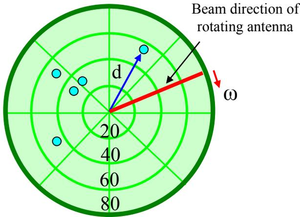
**Fig. 8.5:** A PPI display: the antenna beam direction is shown by the radial bar which rotates in synchronism with the antenna. Dots represent target positions. Numbers on the circles indicate their radial distances from the antenna.
