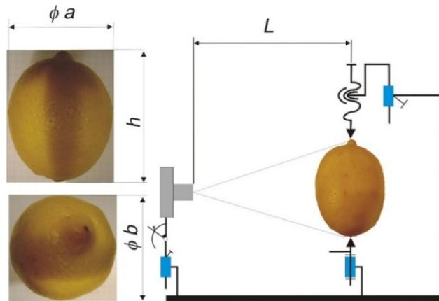
Figure 1. Symbols of basic dimensions of lemons and a test stand
