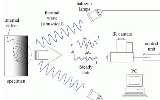
Fig. 2. Schematic view of thermal excitation – enforce LockIn[5]
