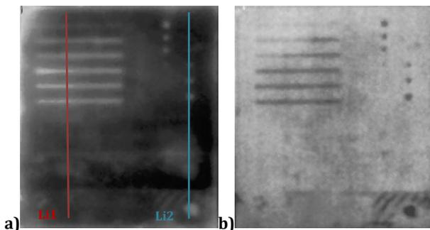
**Fig. 5. The thermal image of measured sample: a) LockIn method ; b) Pulse method**
