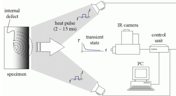
Fig. 1. Schematic view of thermal excitation – enforce Pulse[5]
