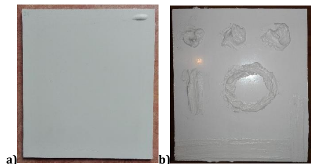
Fig. 8. The view of tested sample; PVC material: a) The real view of the surface of the sample; b) the defect of glue joint
