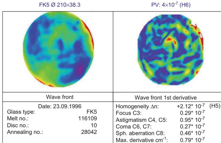
**Figure 2** Optical glass blanks for use as lenses in microlithography are specified with extremely narrow tolerances. With simultaneous development of melting and measurement technologies it became possible to deliver thousands of large blanks with extreme homogeneity.
