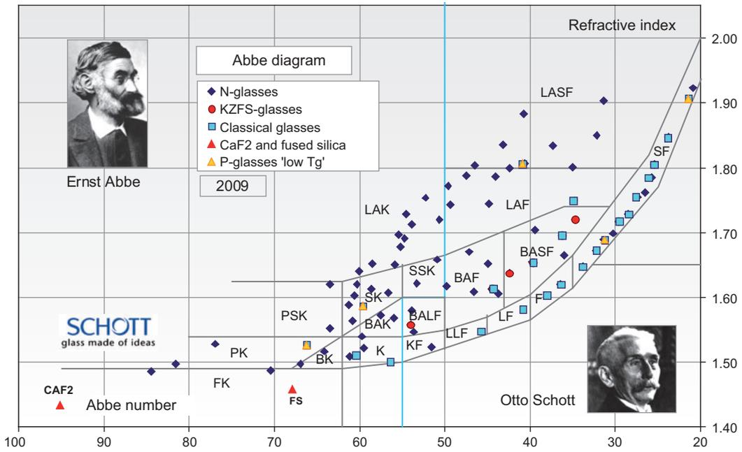
**Figure 1** The Abbe diagram provides an overview for the portfolio of existing glass types plotting their optical positions within the refractive index and dispersion grid. The dispersion is characterized with the Abbe number, which is given traditionally in reverse order as dispersion rises with decreasing Abbe number.
