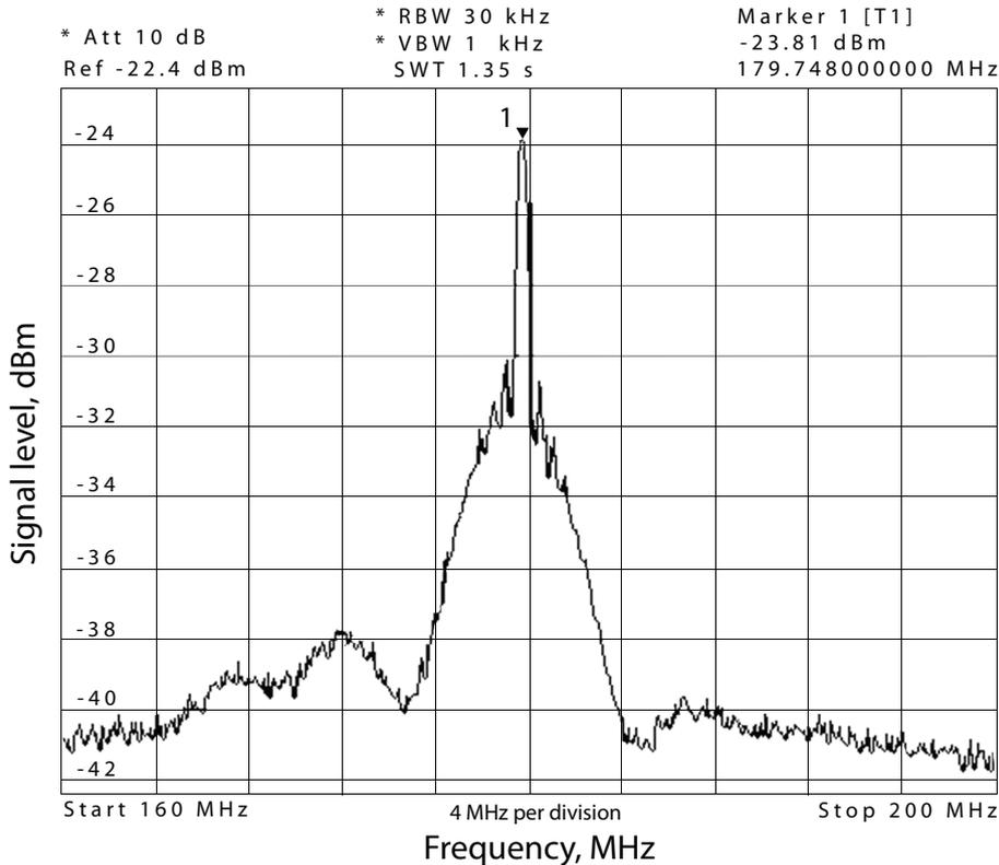
**Fig. 5.** The spectrum of the signal, emitted by a satellite of the navigation system GLONASS, recorded at Irbene after conversion to the intermediate frequency. The central frequency (in MHz) and the level (in dBm) of the signal emitted by the satellite is denoted by a marker 1.
