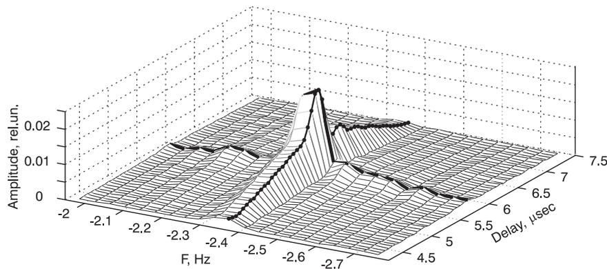
**Fig. 4.** The output signal of the interferometer Irbene–UNN observing the satellite GLONASS ‘37868’.
