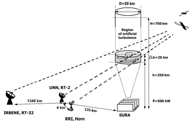
**Fig. 1.** The scheme of VLBI-experiment on receiving the satellite signals which pass through the artificial ionospheric turbulence produced by the heating SURA facility.
