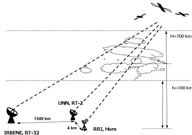
**Fig. 2.** The scheme of the VLBI experiment on radio raying of the ionosphere by a signal of space satellites.
