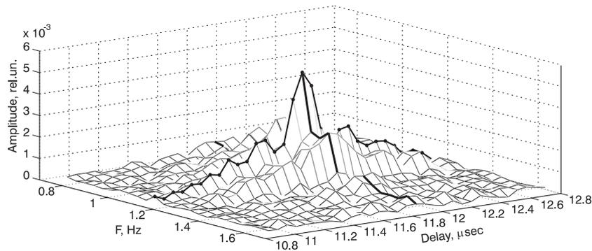
**Fig. 3.** The output signal of the interferometer RRI–UNN for a signal of the satellite GPS ‘26605’. The thin dotted curve denotes cross-correlation function for signals, received in two points of the interferometer; the rich curve shows the power spectrum for the result of multiplication of the signals, recorded with the antennas.
