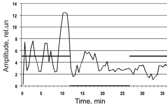
**Fig. 6.** The dependence of amplitude of the interferometer signal on the schedule of SURA during reception of the signal from the satellite NSS GPS ‘26605’; 2012-03-23; the interferometer UNN–RRI.
