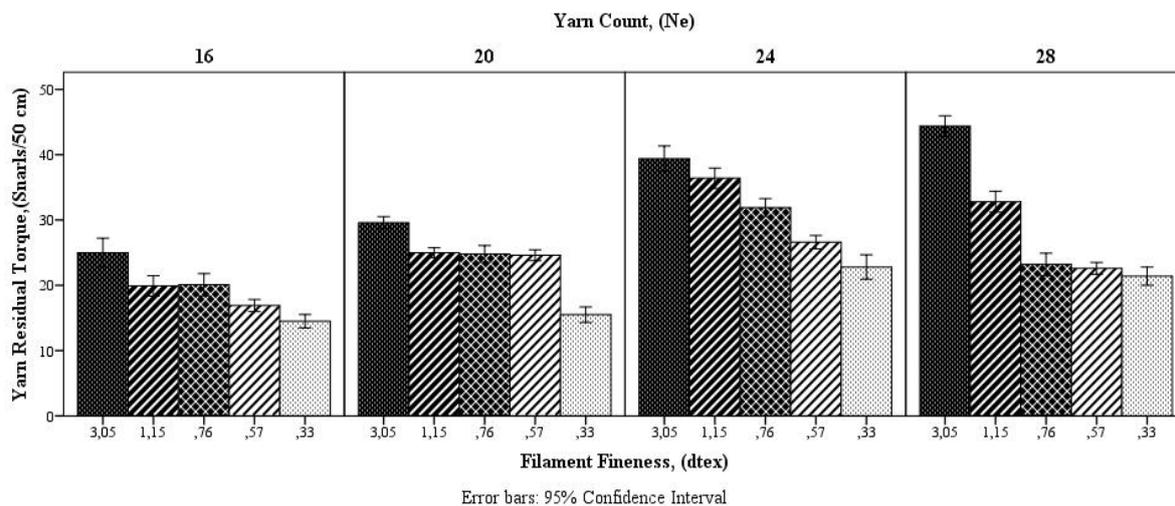
Figure 4. Composite yarn residual torque of samples
