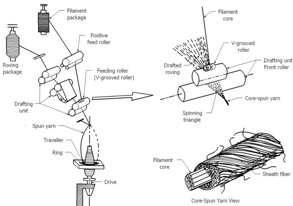
**Figure 2.** Modified ring spinning system, positioning the filament core at the nip point of the front roller, core-spun yarn view (It may not be reproduced without permission)
