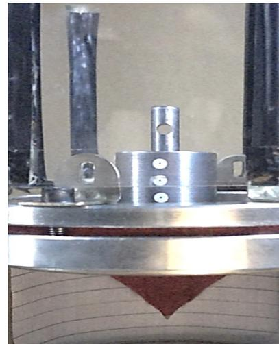
Figure 4. Sample AXβ: The frame captured just at the puncture moment
