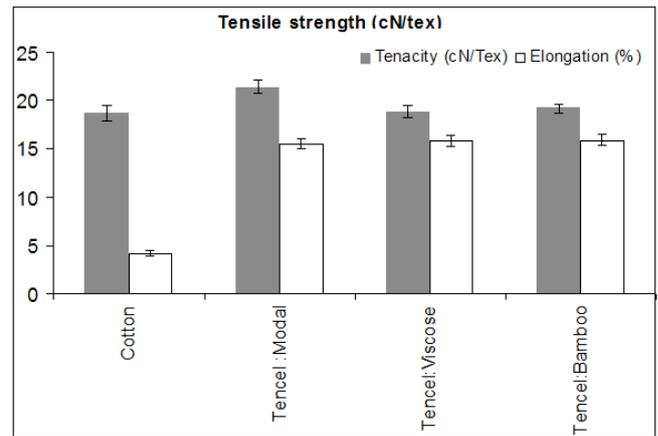
Figure 1. Mechanical properties of yarns
