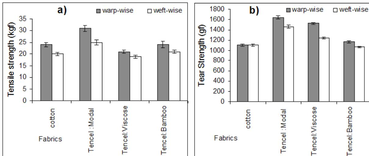
Figure 2. (a) Tensile strength and (b) tear strength of woven fabrics
