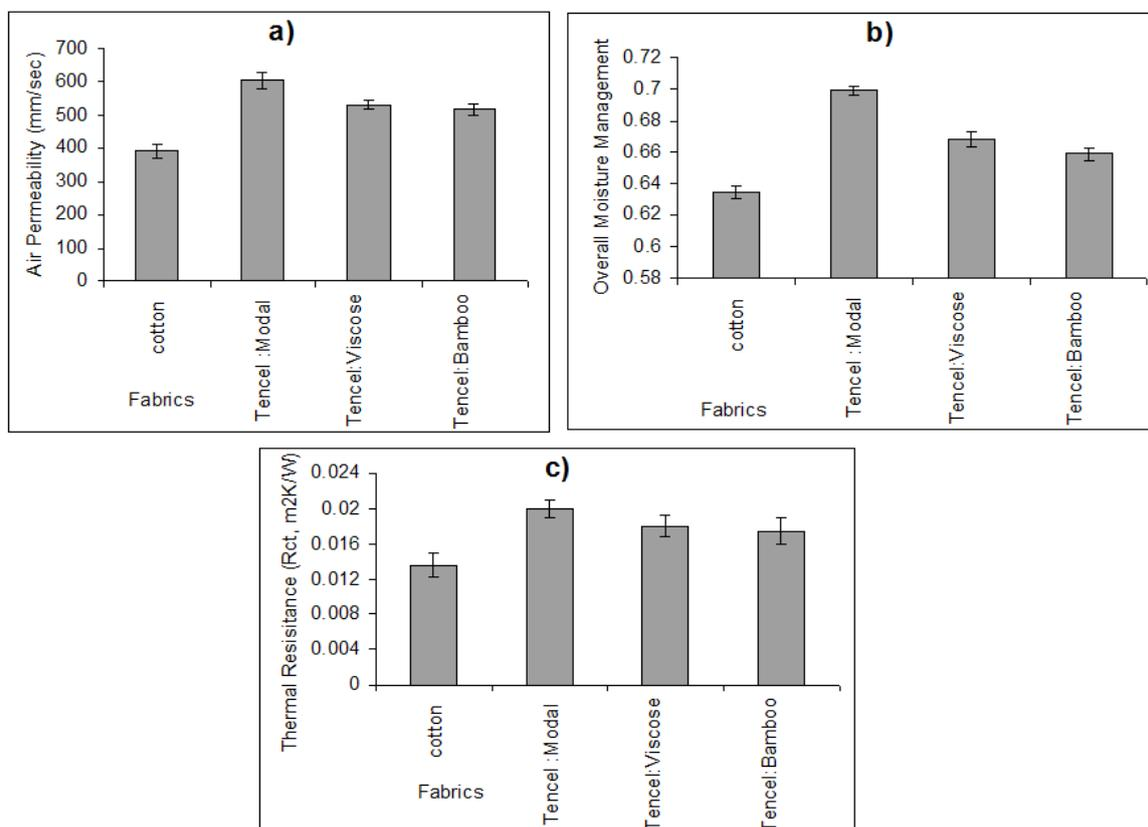
Figure 3 (a) Air Permeability, (b) Moisture Management, (c) Thermal Resistance of fabrics
