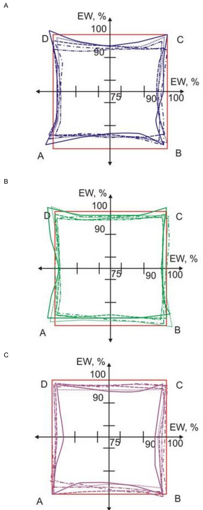
**Figure 2.** The contour width of the embroidery element  $EW$ , accomplished on: a, fabric A1; b, on fabric A2; c, on fabric A3, when the designed contour width of the element ———, 6 mm; ······, 10 mm; - - - - - , 14 mm; - · - · - · , 18 mm; - · - · - · , 22 mm; ———, the contour width  $EW$  of the designed element
