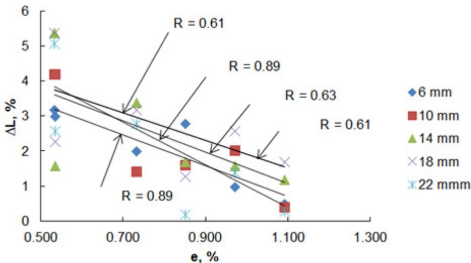
**Figure 3.** The dependency of contour width changes of the embroidery element  $\Delta L$  (%) on the indexes of fabric filling  $e$  (%), when the contour width of the embroidery element EW is as follows:  $\blacklozenge$ , 6 mm;  $\blacksquare$ , 10 mm;  $\blacktriangle$ , 14 mm;  $\times$ , 18 mm;  $\star$ , 22 mm
