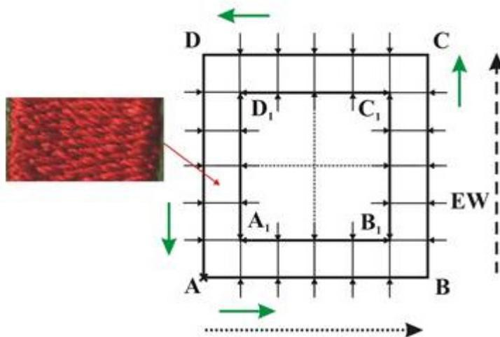
**Figure 1.** The measurement scheme of contour width of the embroidery element; EW, the contour width of the embroidery element; A, the start and end points of the embroidery process; embroidery process direction,  $\rightarrow$ ; fabric threads warp,  $\dots\dots\dots$ ; fabric threads weft,  $- - - -$
