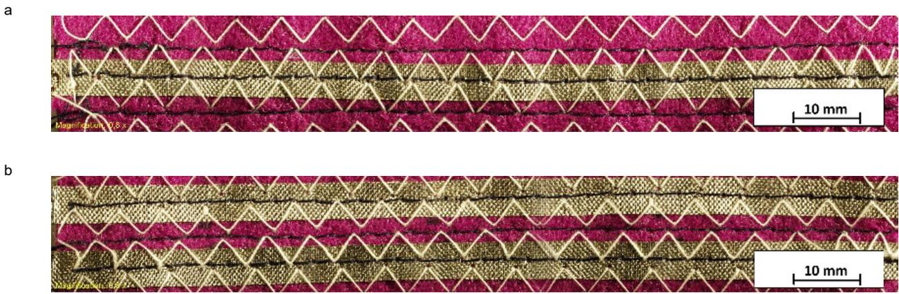
**Figure 1.** Example of the construction of the line being the object of research: a) view from the signal path side, b) view from the path of the mass side [11]
