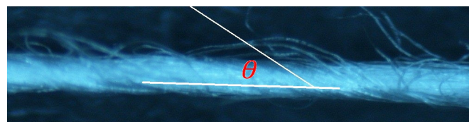
Figure 7. The surface structure of 19.4 dtex jet vortex spun yarn.
