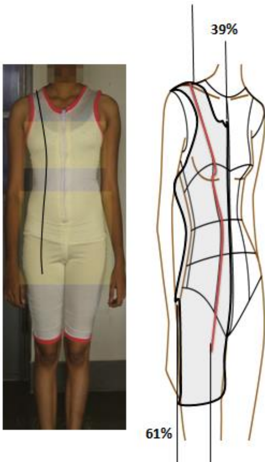
Figure 4. Proportional distribution of pattern segments at the intersection of front shoulder waist line and bust contour line.
