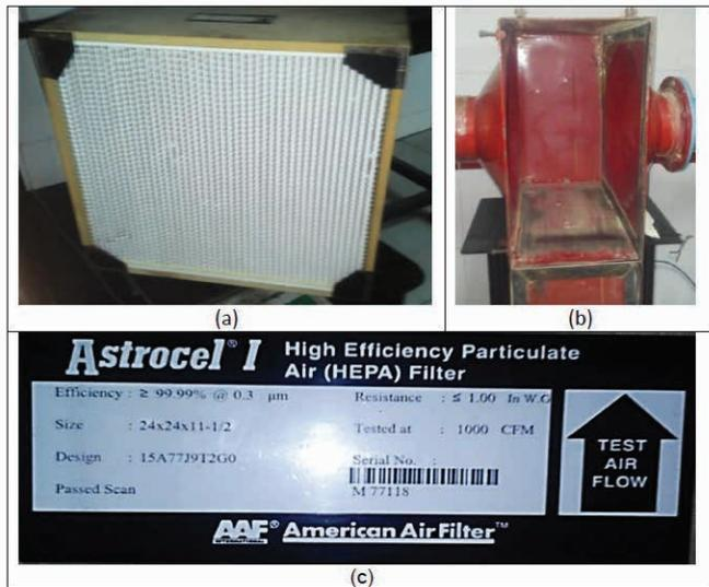
Figure 2.2. The absolute filter construction (a), open housing (b) and its label (c).
