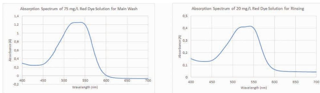
**Figure 3.** Absorption spectra of the Red dye solution for Step 2: (A) main wash and (B) rinsing.
