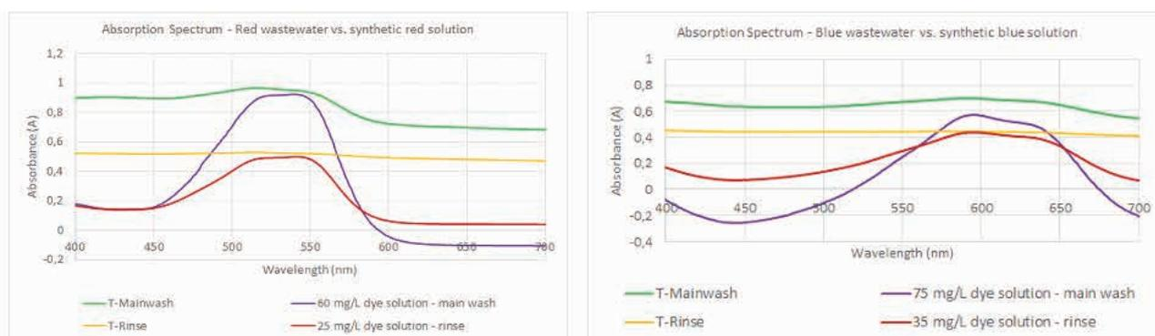
**Figure 5.** Absorption spectra of wastewater versus synthetic dye solutions (A) Red and (B) Blue.
