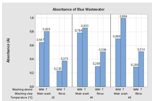
Figure 8. The absorbance values of the wastewater solutions released from the blue fabrics.
