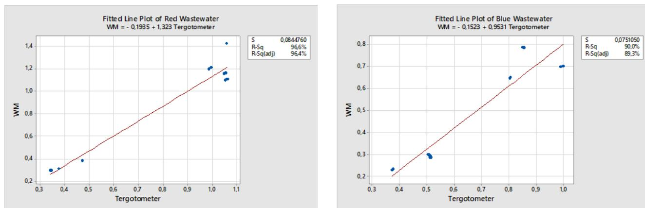
Figure 9. Correlation analysis between the washing machine and tergotometer for the red and blue wastewater solutions.
