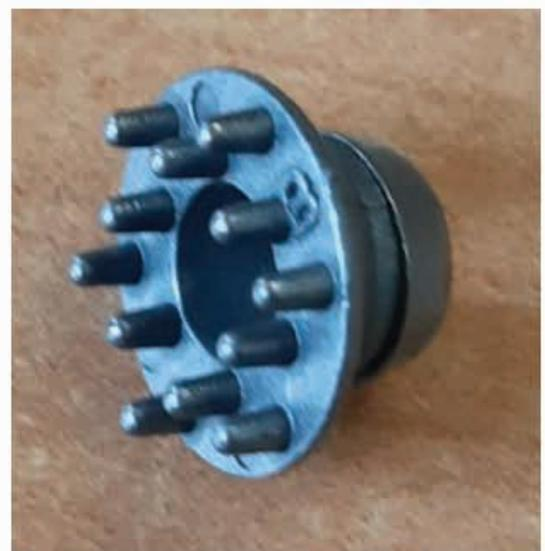
**Figure 3.** Standard EEG electrodes; gold cup wet electrode (left); and pin-shaped dry Ag/AgCl electrode (right).
