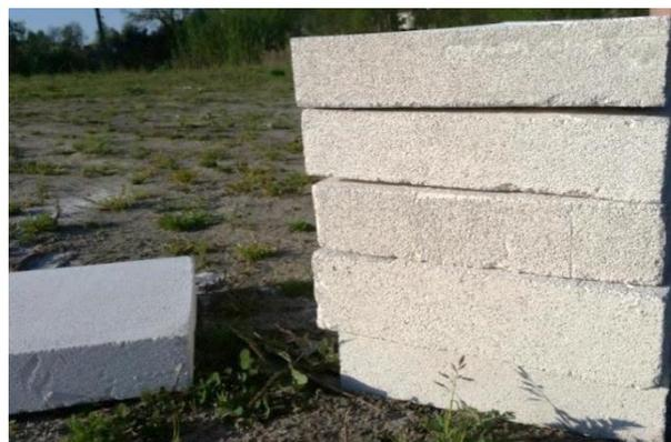
**Fig. 6.** Aerated concrete block samples for thermal conductivity test:
