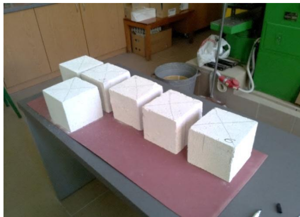
Fig. 5. Aerated concrete block samples for compressive strength test: Aeroc Classic 300 and RocLITE UNIVERSAL 300.
