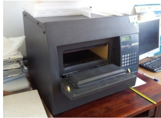
Fig. 4. Heat Flow Meter Netzsch HFM. 436/3/1 E Lambda.
