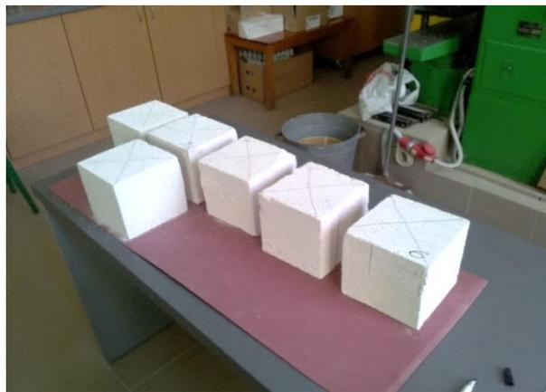
**Fig. 5.** Aerated concrete block samples for compressive strength test:
