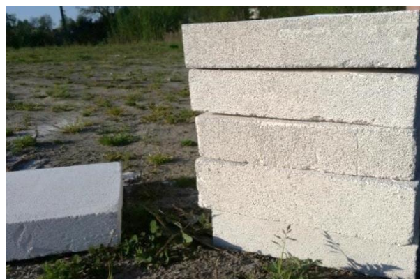
Fig. 6. Aerated concrete block samples for thermal conductivity test: Aeroc Classic 300 and RocLITE UNIVERSAL 300.
