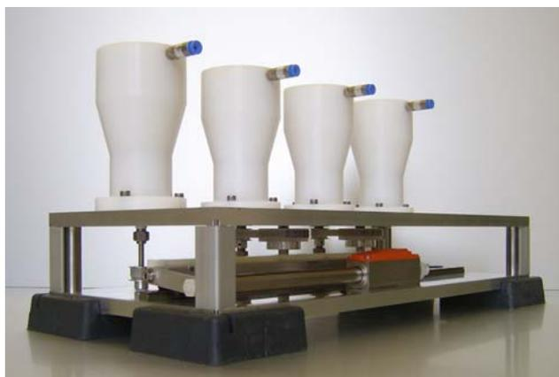
Image 4: Device w/o housing, view to motor and gear
