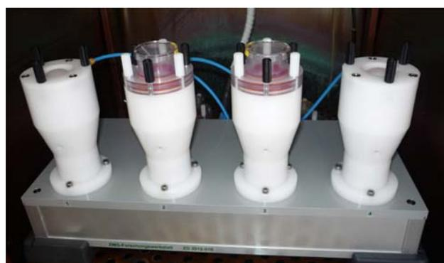
Image 5: *Strain Cell Culture Device* inside the incubator
