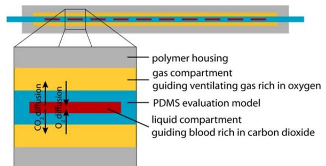
**Image 1:** Schematic of the cross section through the evaluation models mounted in the housing for the experimental setup.
