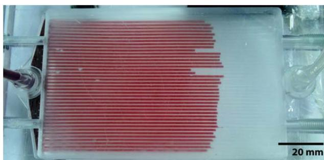
**Image 5:** Filling of the evaluation model with bovine blood. The evaluation model is mounted in the housing, which serves as gas compartment. The filling is homogeneous except for three channels which are partially blocked by entrapped air bubbles.
