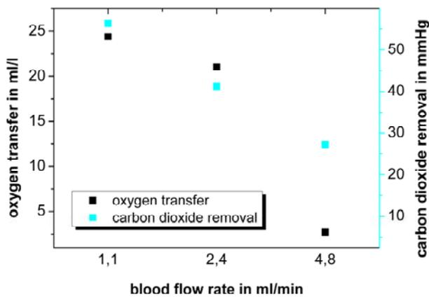
**Image 6:** Gas exchange of an evaluation model with a membrane thickness of 151  $\mu\text{m}$ . Heparinized bovine blood served as a test liquid. The gas exchange was measured for a variation of blood flow rates.
