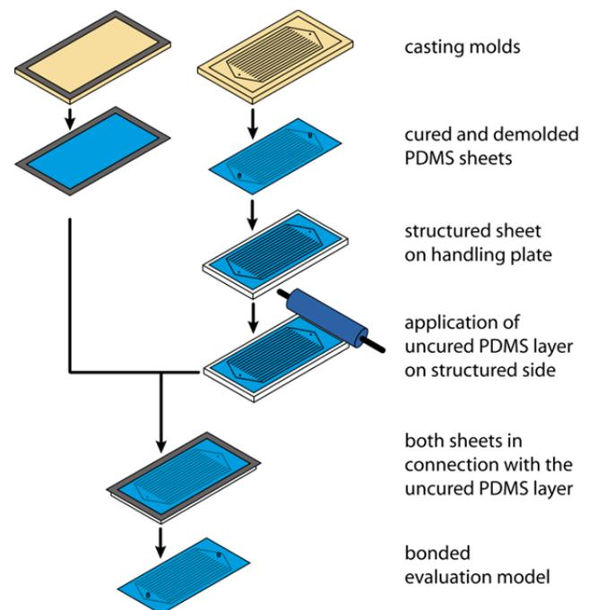
**Image 2:** Fabrication chain of the evaluation models.
