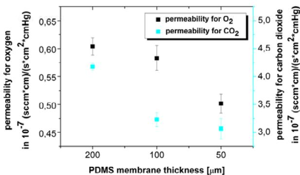
**Image 7:** Measured permeability for oxygen and carbon dioxide of PDMS membranes with thicknesses of 200, 100 and 50  $\mu\text{m}$ .
