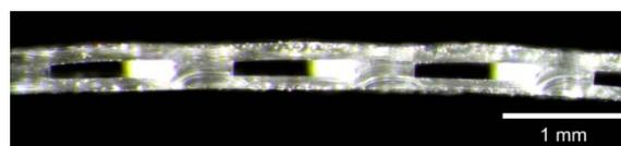
**Image 4:** Cross section through 4 of the 40 parallel micro channels of one evaluation model with a mean membrane thickness of approx. 100  $\mu\text{m}$ .
