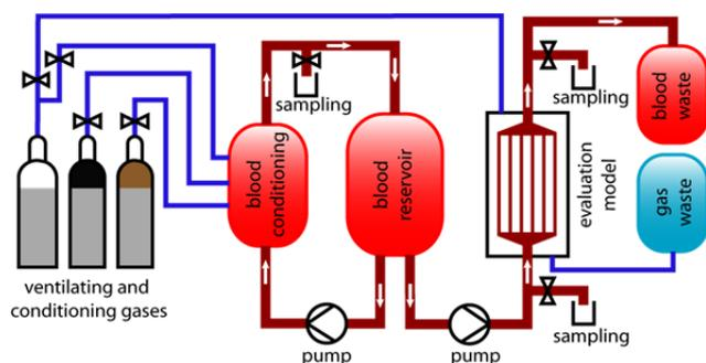
**Image 3:** Schematic of the experimental setup for the gas exchange characterization of the evaluation models.
