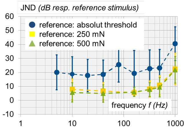
Figure 1: Just noticeable differences for human force perception measured with respect to three different reference stimulus intensities. Results are based on experiments with 36 (250 and 500 mN reference) and 29 test subjects (absolute threshold reference). They comply with Weber's Law, stating higher JNDs when reference stimuli approach the absolute perception threshold.
