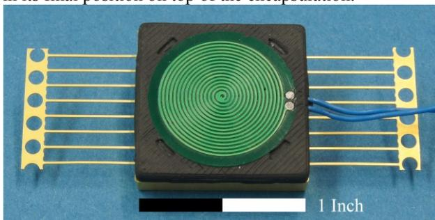
Figure 1: Ferrite cover containing coil on top of the ferromagnetic metal housing
