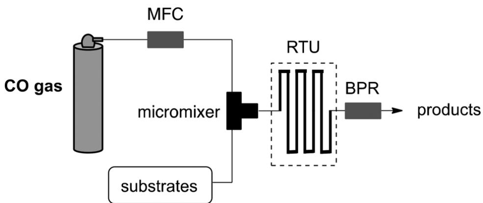
**Figure 3:** Typical flow reactor system for carbonylation (MFC: mass flow controller; RTU: residence time unit; BPR: back pressure regulator). With permission from reference [17] (license number: 3701431434096).
