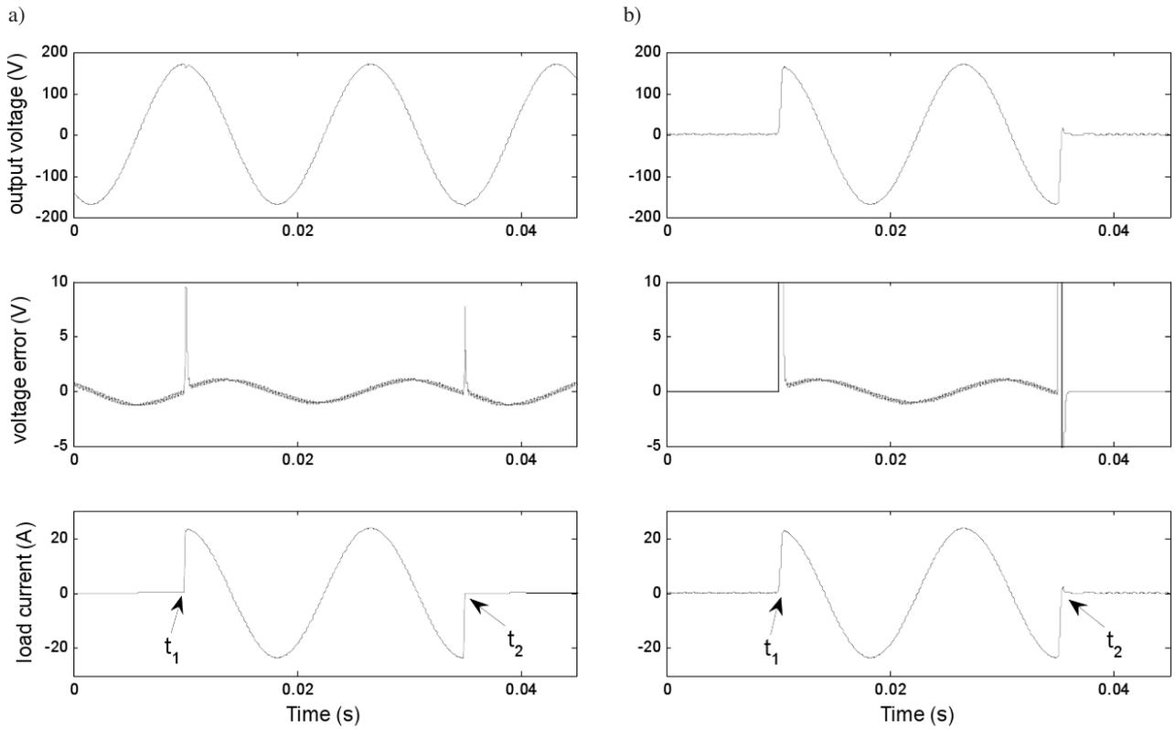
Fig. 8. Transient waveforms: a) 100% application (at  $t_1$ ) and 100% removal (at  $t_2$ ) of load, and b) 100% jump (at  $t_1$ ) and 100% fall (at  $t_2$ ) of reference voltage
