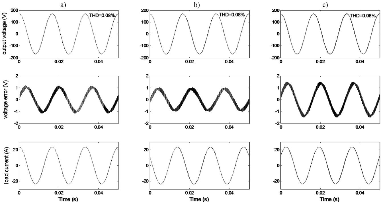
Fig. 4. Steady-state waveforms under (a) unity, (b) 0.5 leading, and (c) 0.5 lagging power factor load
