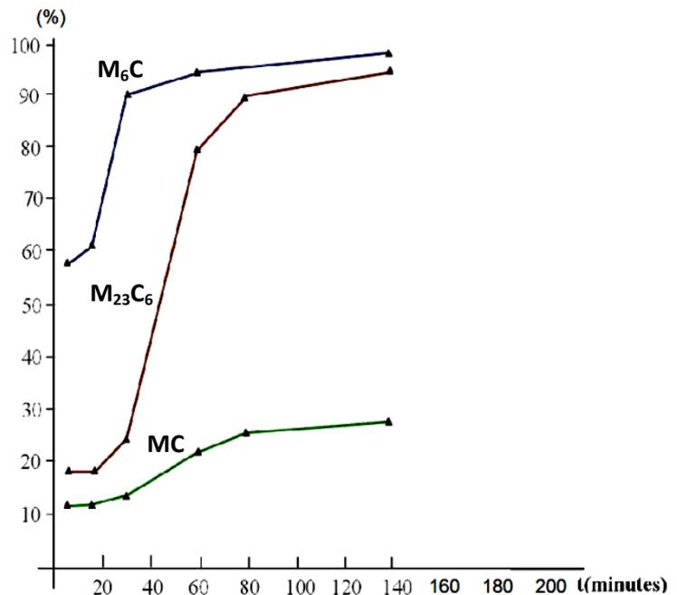
Figure 6. The curves depicting the kinetics of precipitated carbides
