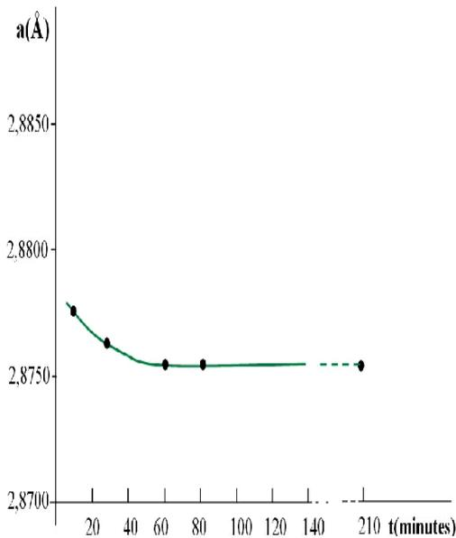
Figure 5. The martensite lattice parameter variation according to the time of tempering
