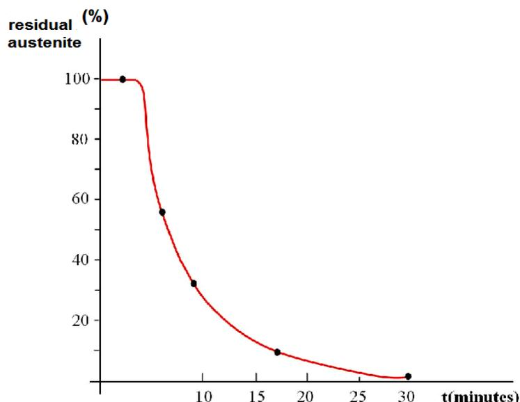
Figure 4. Kinetics curve for transformation of residual austenite
