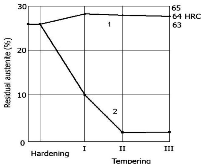
Figure 2. Variation of hardness and the amount of residual austenite on the tempering at 560<sup>0</sup> C [8]
