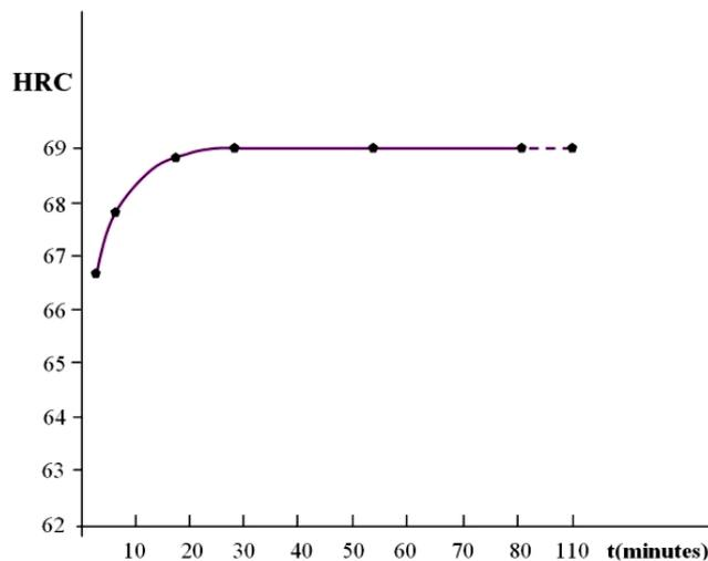
Figure 7. The maximum hardness of investigated steel
