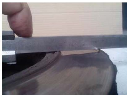
Figure 5. Irregular worn-traces on disk left by brake plate
