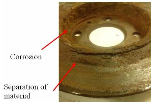
Figure 3. Macrostructural appearance of the used brake disc
