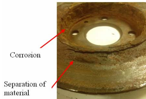
Figure 3. Macrostructural appearance of the used brake disc
