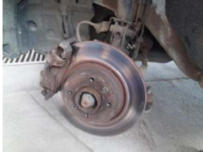
Figure 4. Irregular worn disc with blue spots
