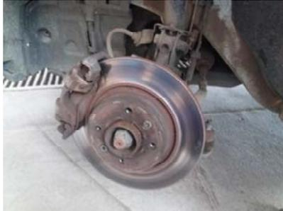
Figure 4. Irregular worn disc with blue spots
