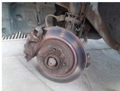
Figure 4. Irregular worn disc with blue spots
