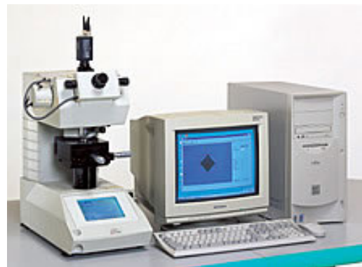
Figure 2. Automatic reading system for Vickers hardness tests
