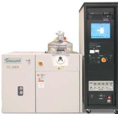
**Figure 1. System of deposition by electrons beam evaporation Temescal FC-2000 [7]**
