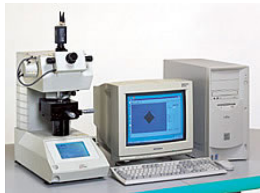
Figure 2. Automatic reading system for Vickers hardness tests
