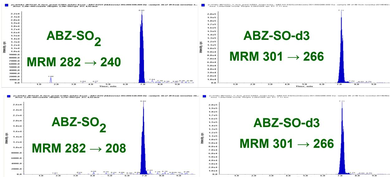
**Fig. 1.** The ion chromatograms of the incurred goat milk containing albendazole sulfone (5.2 µg/kg). The chromatograms present two transitions (MRMs, multiple reaction monitoring) of albendazole sulfone ( $m/z = 282$ ) in comparison to ion chromatogram of a labelled internal standard (albendazole sulfone – d3)
