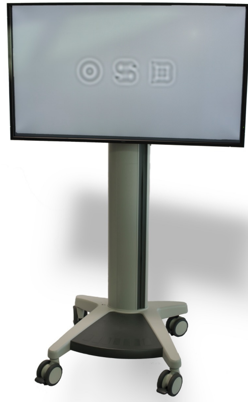
Figure 1: Picture of a device prototype in demo mode, where particularly visible (medium spatial frequency, high contrast) stimuli are shown.
