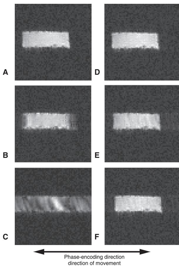
**Figure 4:** Images ( $64 \times 64$ ) of the agarose cylinder: (A) no motion (B) periodical movement (C) gated with periodical movement and without phase correction (D) gated with periodical movement and phase correction (pos. 0 mm) (E) gated with periodical movement and phase correction (pos. 1 mm) (F) gated with periodical movement and phase correction (pos. 2 mm).
