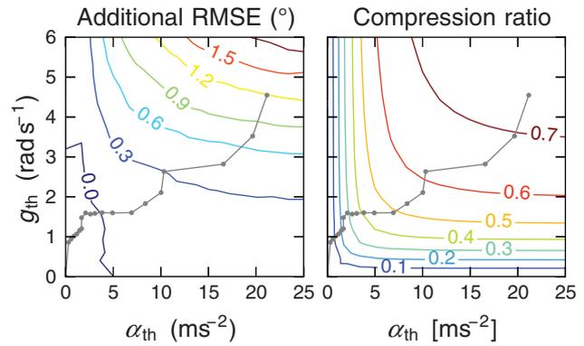
**Figure 2:** Contour plot showing the additional RMSE (i.e. the RMSE obtained with event-based sampling minus the RMSE obtained with full sampling) and the compression ratio obtained using Method 2 when varying the two thresholds  $\alpha_{th}$  and  $g_{th}$ . The gray line shows the trajectory used to generate the respective curve in Figure 3.
