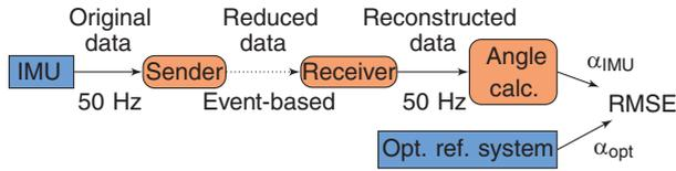
**Figure 1:** Online event-based sampling is simulated by using recorded IMU data as input to an event-based sender. The receiver reconstructs the data, which is fed to the angle calculation algorithm and the results are compared to angles obtained by optical motion analysis.
