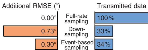
**Figure 4:** Compared to standard full-rate sampling, send-on-area sampling with decreasing thresholds (Method 4) can reduce the transmitted data by 66% while increasing the total average RMSE by only 0.3°.
