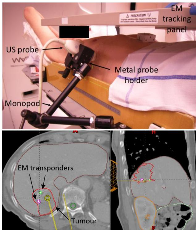
**Figure 1:** Top – Setup for simultaneous acquisition of 4D ultrasound imaging and electromagnetic tracking. The ultrasound probe was attached to the patient couch to continuously visualize the target region. Bottom – Two (out of three) implanted transponders in the liver surrounding the tumour.
