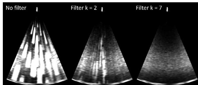
**Figure 2:** Effect of Calypso signal on ultrasound images (left) and result of an increasing amount of temporal filtering ( $k = 2, \dots, 7$ ).
