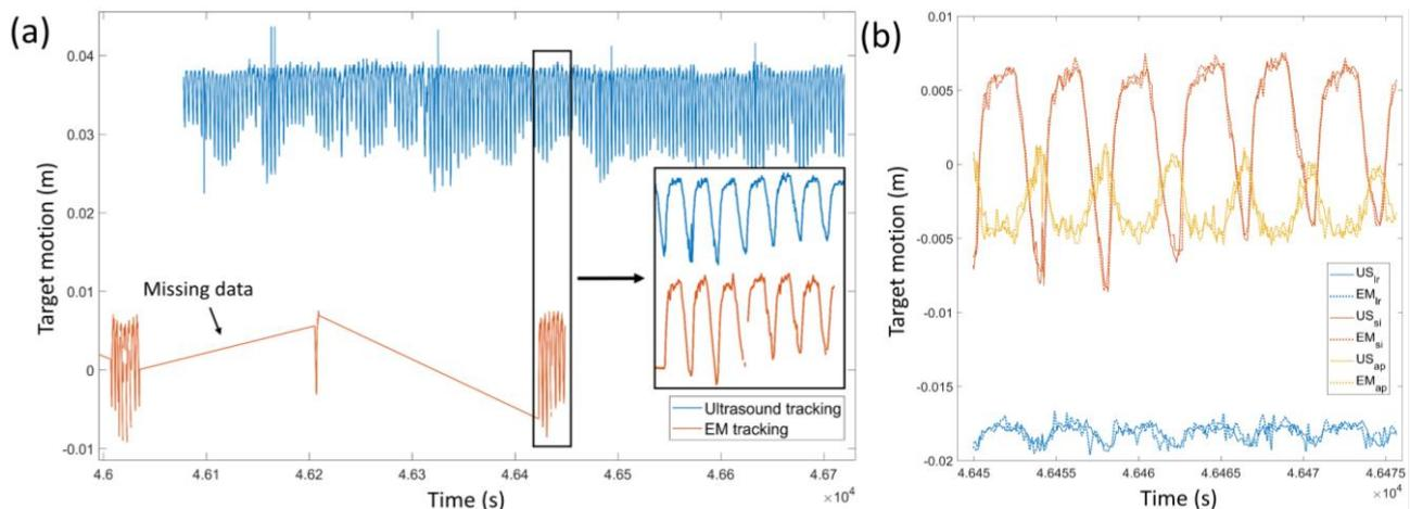
**Figure 4:** (a) Temporal synchronization of ultrasound and EM tracking data. Interference from metal components disturbed the EM tracking system, leading to missing data points. (b) The spatially aligned transponder trajectories measured with ultrasound and EM tracking.
