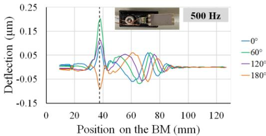
**Figure 4:** The BM oscillation for IC stimulation at  $f=500\text{Hz}$  for different phases.
