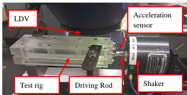
**Figure 1:** The experimental setup characterization of the test rig with respect to its tonotopic character.
