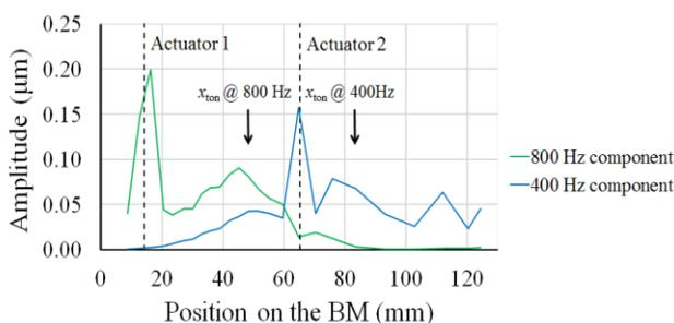
**Figure 7:** Dual actuator stimulation: BM oscillation envelope curves for simultaneously driven piezoelectric actuators when stimulating actuator 1 with  $f=800$  Hz and actuator 2 with  $f=400$  Hz. The grey dashed lines mark the position of the piezoelectric actuators.
