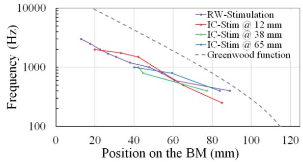
**Figure 5:** The tonotopic character of the test rig for RW and IC stimulation. Dashed line: Greenwood function describing the human cochlea adapted to our membrane length.
