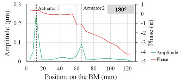
**Figure 6:** Dual actuator stimulation: BM oscillation envelope curves with simultaneously identical frequency driven piezoelectric actuators when stimulating with  $f=400\text{Hz}$  for different phases and the corresponding phase response. The grey dashed lines mark the position of the piezoelectric actuators.
