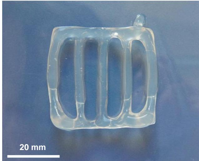
**Figure 4:** Printed scaffold with simple gridline structure after ionically crosslinking in bath of 5% w/v aqueous solution of  $\text{CaCl}_2$ .
