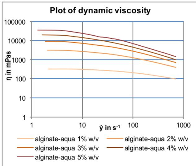
**Figure 2:** Logarithmic plot of dynamic viscosity  $\eta$  over shear stress  $\dot{\gamma}$  ( $T=20^\circ\text{C}$ ). All solutions show shear thinning behaviour.
