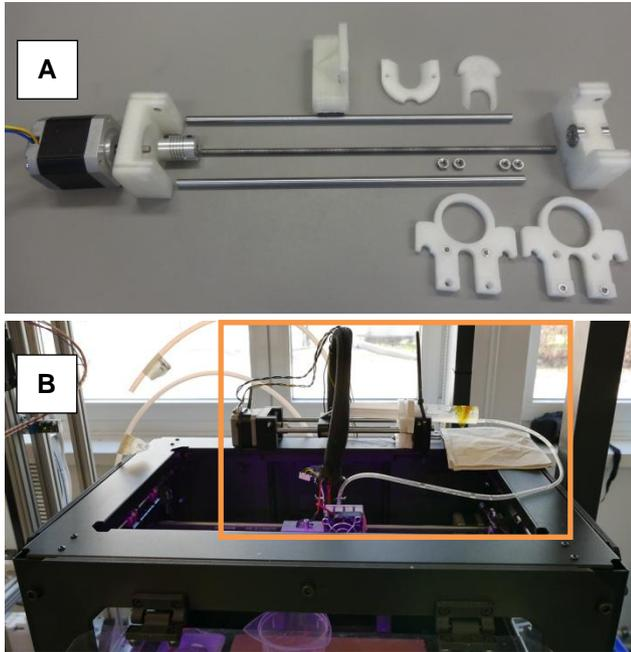
**Figure 1:** (A) 3D-printed syringe pump by Wjien et al. [5] (printed parts are white) and (B) printer setup of this work using Makerbot Replicator 2X equipped with 3D-printed syringe pump (marked).
