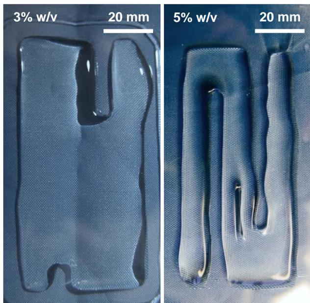
**Figure 3:** Exemplary pictures of printed z-shaped test-structures (not crosslinked). The printing of more viscous alginate solutions results in increasing accuracy of printing performance.
