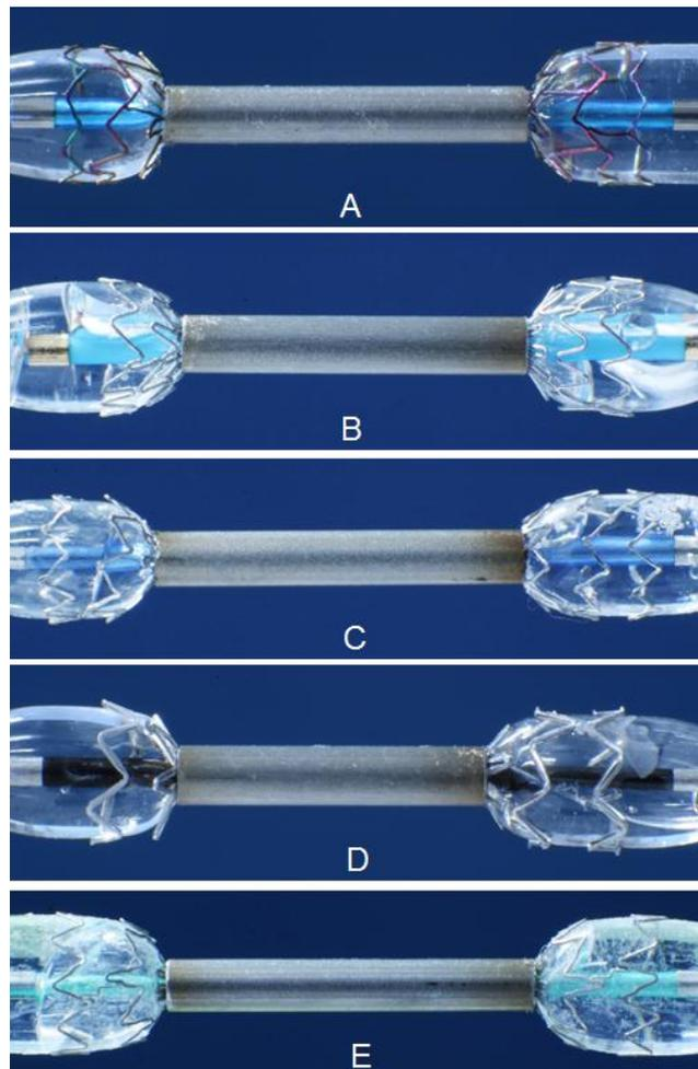
**Figure 1:** Expanded stents at RBP in the resistant focal stenosis model – A) Synsiro 3.0/15, B) Resolute Integrity 3.0/15, C) PROMUS Element Plus 3.0/16, D) BIOMATRIX Neoflex 3.0/14, E) Coroflex ISAR 3.0/16
