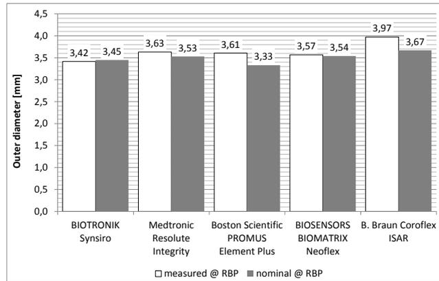
**Figure 4:** Measured maximum outer diameters compared to nominal outer diameters (corrected by stent wall thickness) at RBP
